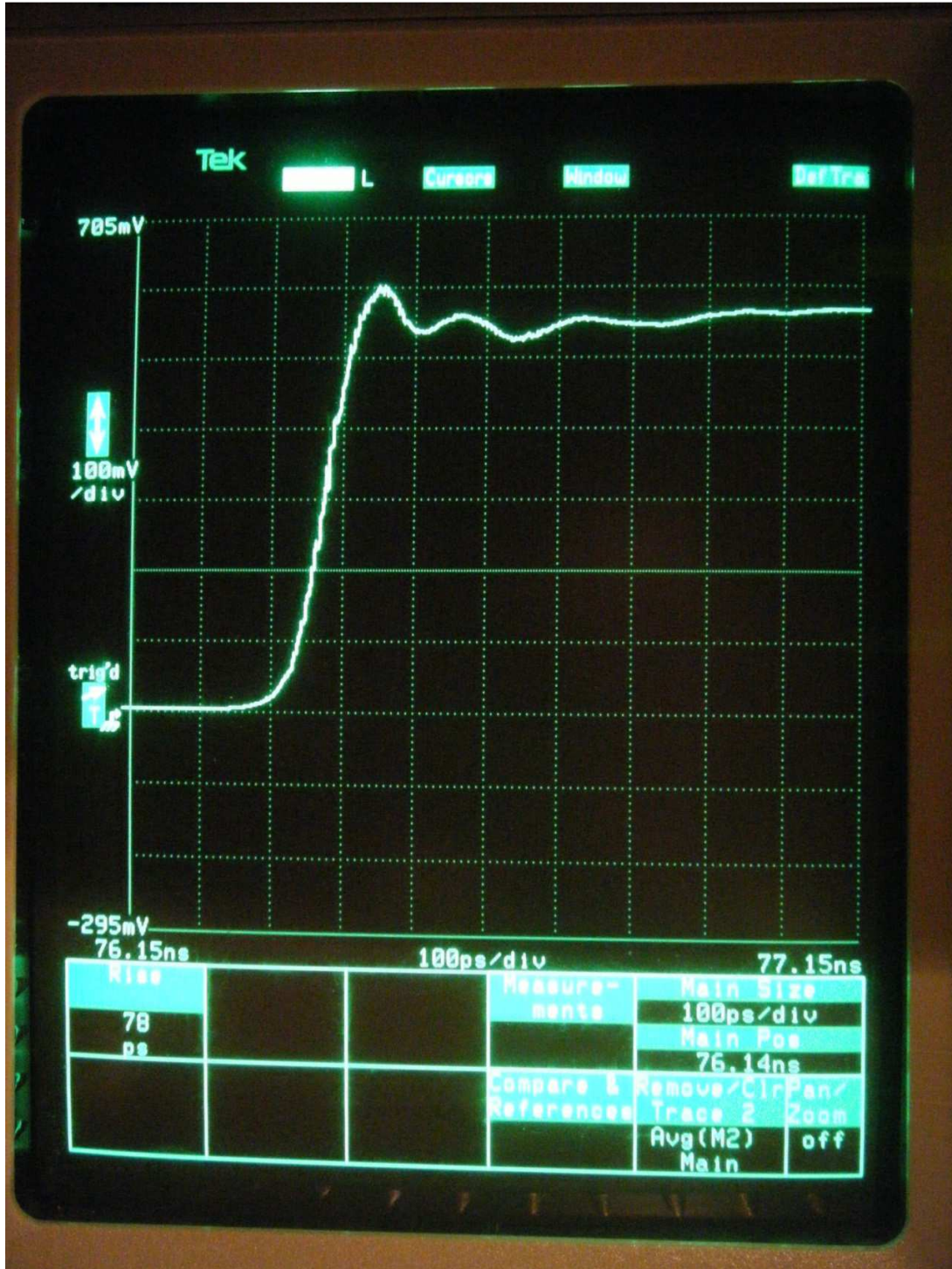
Picture 3 - Measured with Tektronix SD-24 in 11801 mainframe 20 GHz sampling scope. Risetime 100ps/div Measured risetime is 78ps (light travels 25 mm in 78ps, a signal on the board about 17mm)
