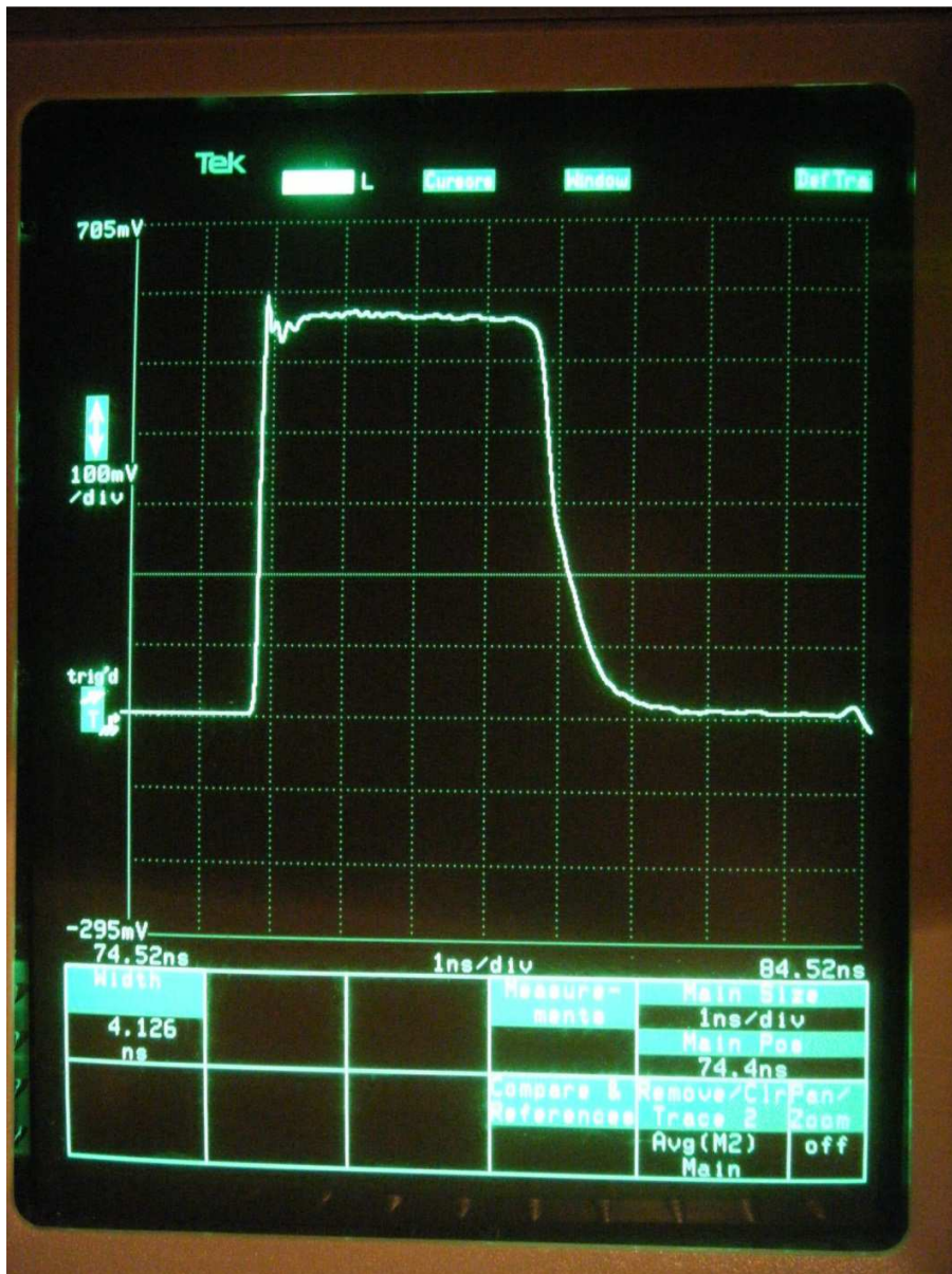
Picture 1 - Measured with Tektronix SD-24 in 11801 mainframe 20 GHz sampling scope. Full pulse 1ns/div
