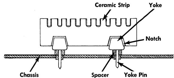
Fig. 1-2. Ceramic terminal strip installation.
