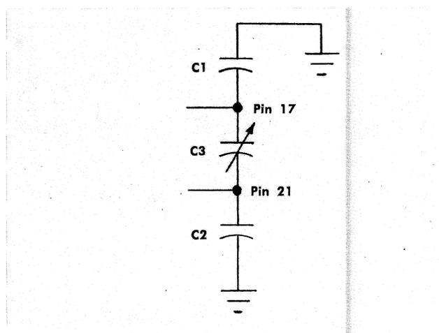
Fig. 2-2. Schematic representation of effective deflection-plate capacity.
