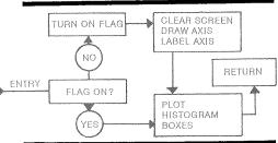
If the flag is "off" the first time the subroutine is called, the calculator will put Part A in operation. This action clears the screen, establishes the X and Y axis, labels them and then turns on the flag. Your calculator then executes Part B, the only section necessary in subsequent use of the subroutine. Upon its completion, your calculator returns to the main program.
