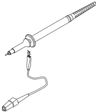
**Ground Lead.** Use the alligator clip to attach the probe to a ground reference.
