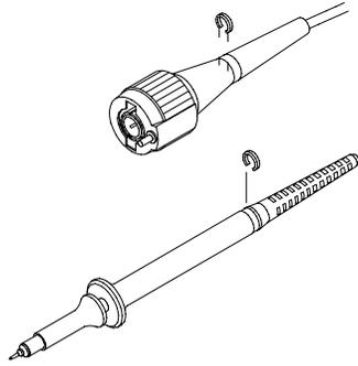
**Marker rings.** Attach the matching colored rings onto the probe cable and tip as shown.
