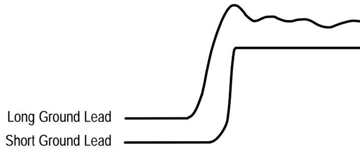
To see the best signal, use the shortest possible ground lead and signal path.
