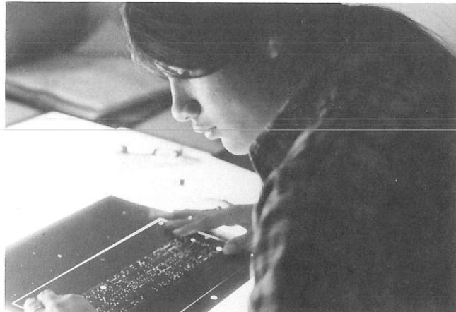
Juanita Orozco aligning the front and back filmwork for a pc board.
