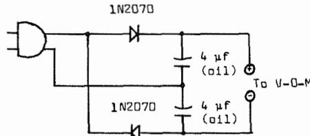
Figure C. Peak-to-peak reading adapter for 20,000  $\Omega$ /volt V-O-M.
