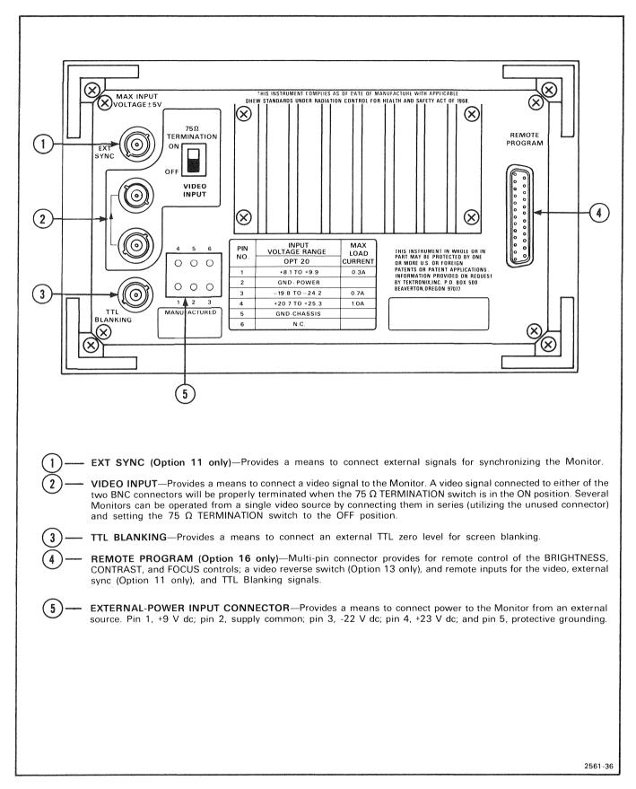
Figure 2-3. Option 20 rear-panel controls and connectors.
