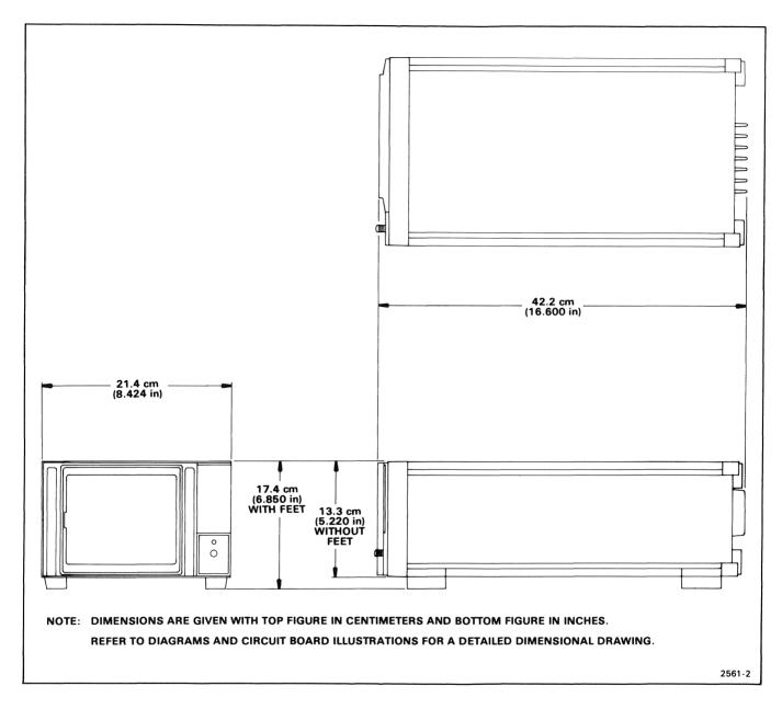
Figure 1-1. Dimensional drawing (Standard instrument package).
