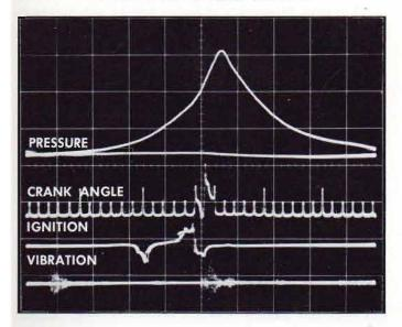
Simultaneous displays of four engine parameters provide the operator with one comprehensive picture of the total engine performance and make identification of malfunctions easy. The top waveform is engine pressure; waveform 2 shows crank-angle markers with the larger marker in the center indicating the top dead center; waveform 3 is engine ignition; waveform 4 is engine vibration showing valves opening and closing and vibration due to combustion.
