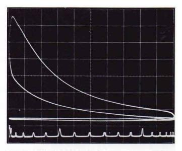
Pressure vs cylinder volume displays are used to determine the indicated engine horsepower and detect over-all problems in engines and compressors. The area within the loop is the mean effective pressure and is used to determine indicated horsepower of the engine.
