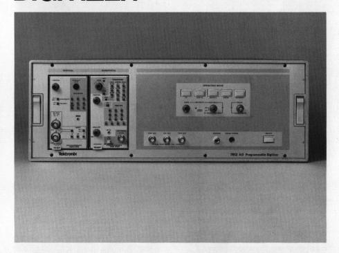
Capturing high-speed waveforms is the 7912AD's forte. Each waveform can be sampled up to 512 times within a selectable time window, ranging from ten milliseconds to five nanoseconds (50 kHz to 100 GHz equivalent sampling rate).
