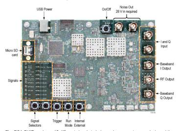
The RSA-DKIT produces 16 different signals to help you learn spectrum analysis and the latest measurement methods.
