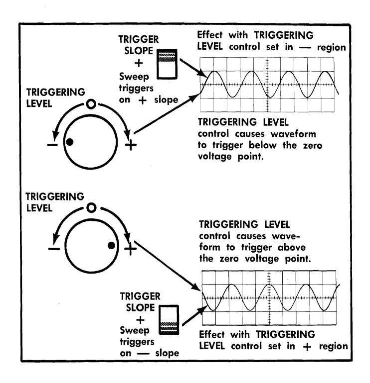
Fig. 1. Effects of the TRIGGERING LEVEL and TRIGGER SLOPE controls.
