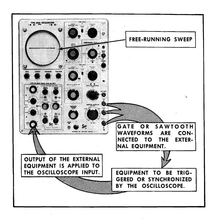
Fig. 2. Using the Gate or Sawtooth output waveforms to synchronize or trigger external equipment.
