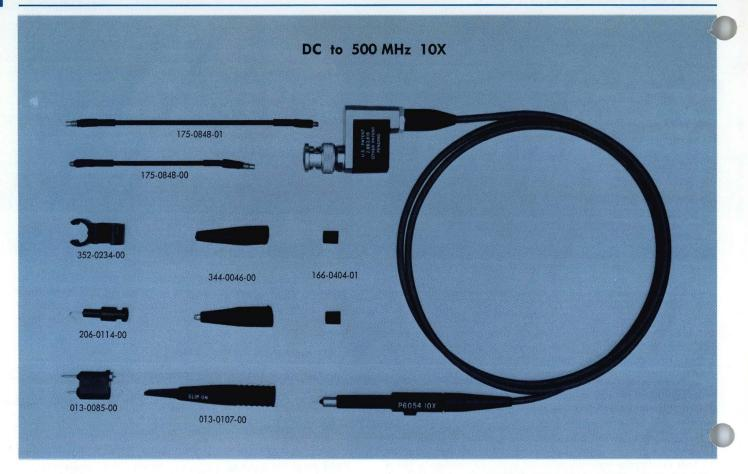
The P6054 is a miniature, fast-rise, 10X probe designed for use in conjunction with Tektronix oscilloscopes having a nominal input capacitance of 15 to 24 pF. The probe does not incorporate CRT readout/trace-identify functions.
