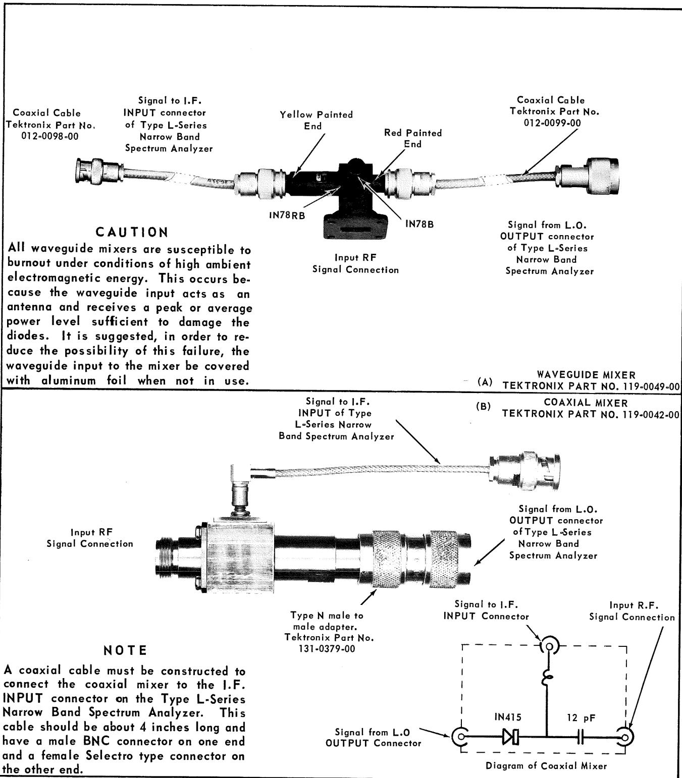
Fig. 1-2. External mixers available for the Type L-Series Narrow Band Spectrum Analyzer which use them. Part (A) shows the external waveguide mixer which is supplied with the L-3852/3 and L-4862/3 Spectrum Analyzers. Part (B) shows an external coaxial mixer which can be used with the L-3852/3 and L-4862/3 Spectrum Analyzers to permit these instruments to be used on their fundamental and 2nd harmonic frequencies.
