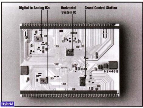
Containing the entire acquisition circuitry for each input channel, this hybrid dramatically increases these scopes' reliability.
