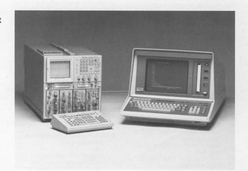
**Data Storage.** Acquired and processed data such as waveforms and calculated results can be stored for future reference using the 4052 mag tape.
