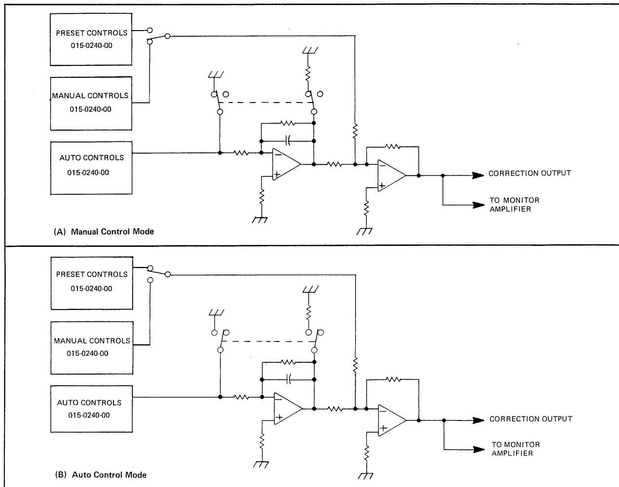
Fig. 1-2. 1440 modes of control. (A) Manual Control Mode (Manual/Preset). (B) Auto Control Mode (VIRS).
