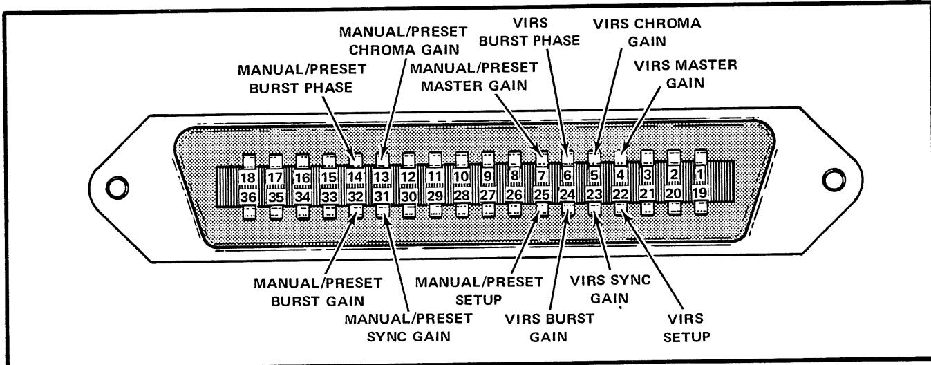
Fig. 1-1. Rear panel connector showing control routing.
