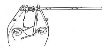
7. Open the jaws of the crimping tool and insert the eyelets in the notches in the tips of the jaws as shown. Squeeze the handles of the tool to compress the eyelets together.
