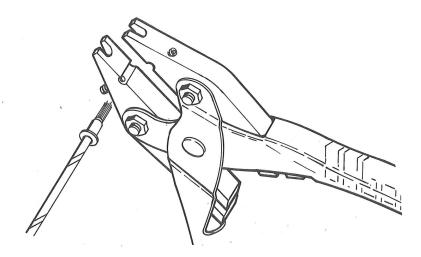
4. Insert the eyelet into the notch in the jaws of the crimping tool, making sure the protruding pins come in contact with the eyelet (if not, turn the tool over). Check the alignment of the eyelet then crimp the eyelet onto the cable.
