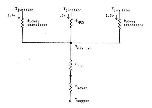
$\theta_{\text{power transistor}}$  = from 30°C/w to 50°C/w depending on device and die bond (measured).
