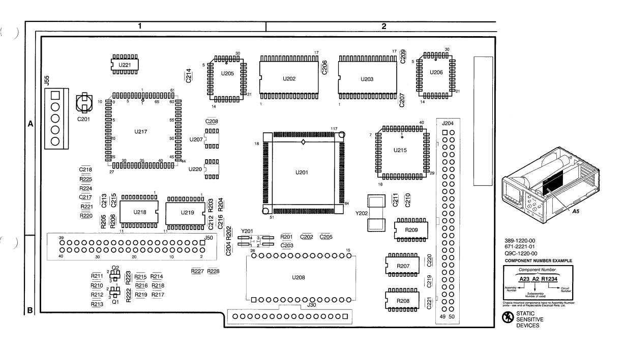
Figure 9-6: A5 Processor Board TAS 455 — SN B011862 and Below TAS 465 — SN B011621 and Below
