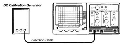
Figure 4-7: Trigger Level Test Setup
