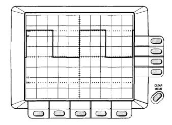
Figure 2-4: Probe Compensation Signal Displayed after AUTOSET
