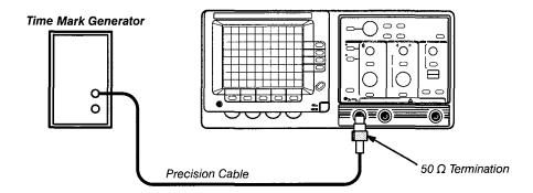
Figure 4-11: Dual Delay Test Setup
