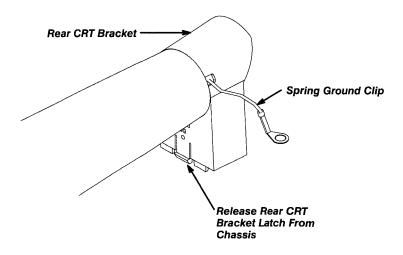
Figure 6-15: CRT Rear Bracket and Ground Clip
