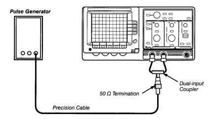
Figure 5-13: Attenuator Compensation Test Setup
