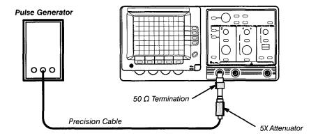
Figure 5-12: High Frequency Step Response Test Setup
