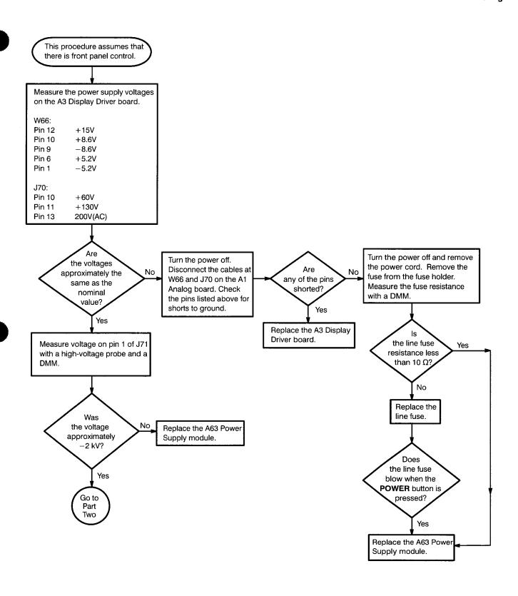
Figure 6-22: A3 Display Driver Board Troubleshooting Procedure
