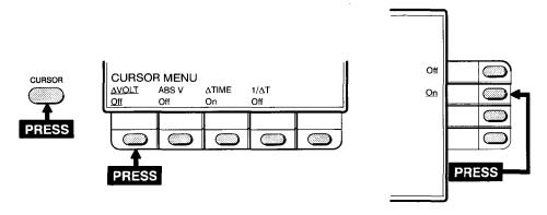
4. Now two horizontal bar cursors are displayed. The active (movable) one is a solid line and the inactive one is a dashed line. Use the General Purpose Knob to move the active cursor and use the **TOGGLE** button to select which cursor is active.
