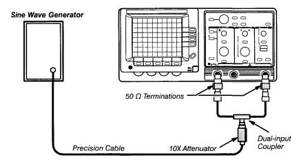
Figure 4-15: Trigger Sensitivity Test Setup Four
