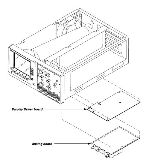
Figure 5-1: Location of Boards for Adjustments
