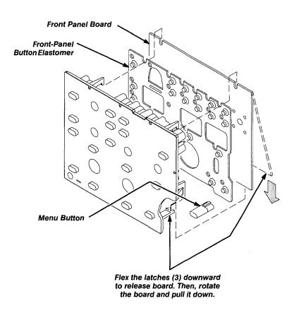
Figure 6-10: Disassembly of Front-Panel Assembly
