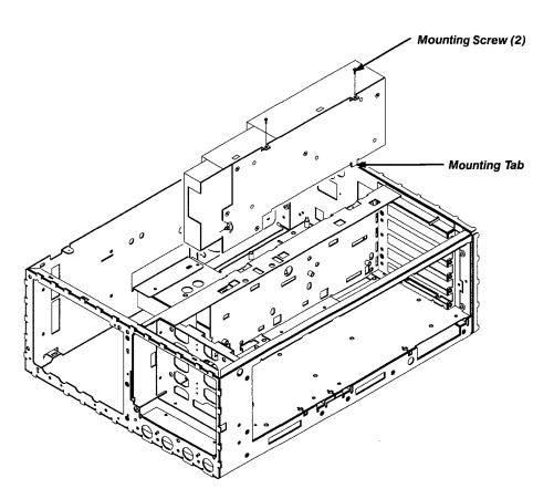
Figure 6-18: Power Supply Removal
