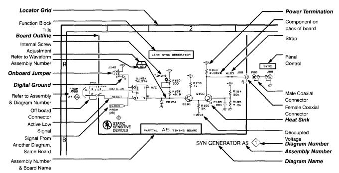
Figure 9-1: Graphic Items and Special Symbols Used in This Manual
