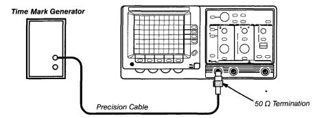
Figure 4-10: Timing Test Setup
