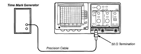
Figure 5-2: CRT Adjustments Calibration Setup
