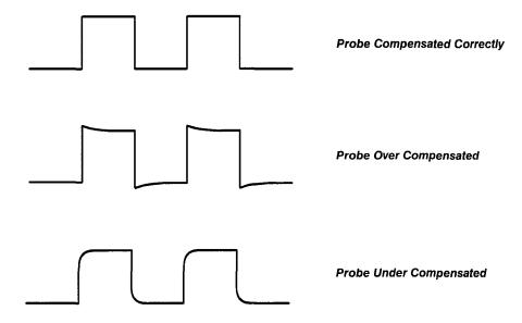
Figure 2-6: How Probe Compensation Affects Signals
