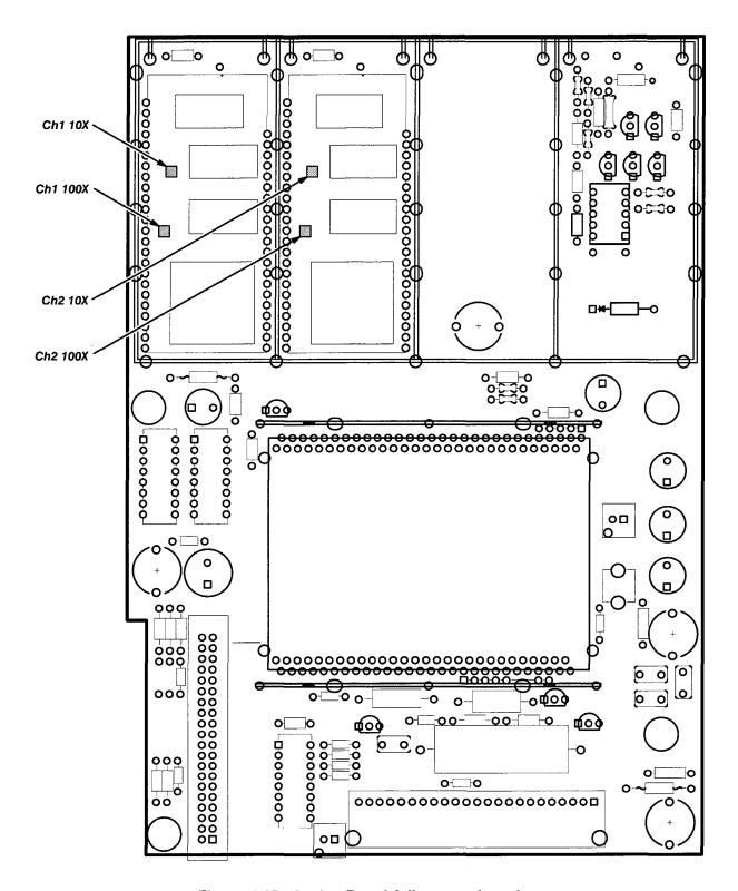
Figure 5-15: Analog Board Adjustment Locations
