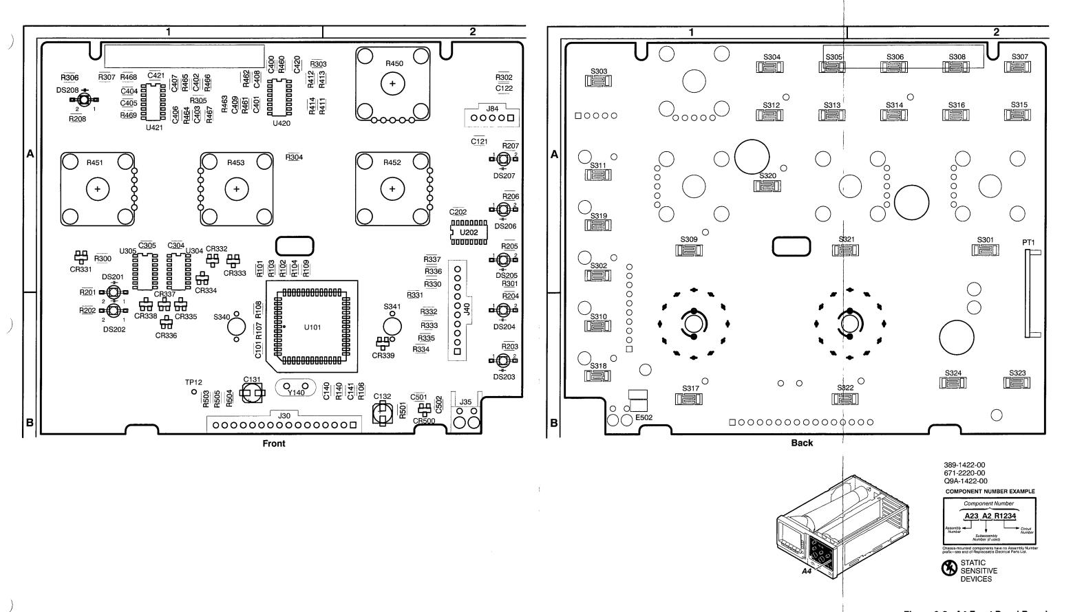
Figure 9-8: A4 Front Panel Board
