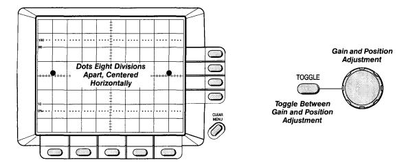
Figure 4-3: Horizontal Adjustments (One)
