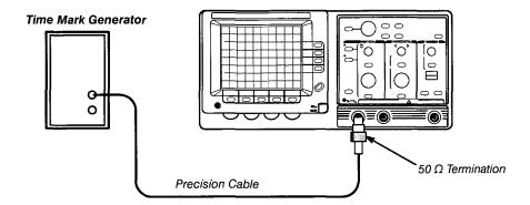
Figure 5-7: Horizontal Output Calibration Setup
