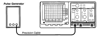
Figure 4-9: X-Axis Gain Test Setup
