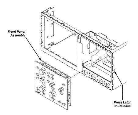
Figure 6-9: A62 Front Panel Module Removal
