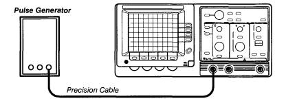
Figure 4-6: Gain and Voltage Test Setup
