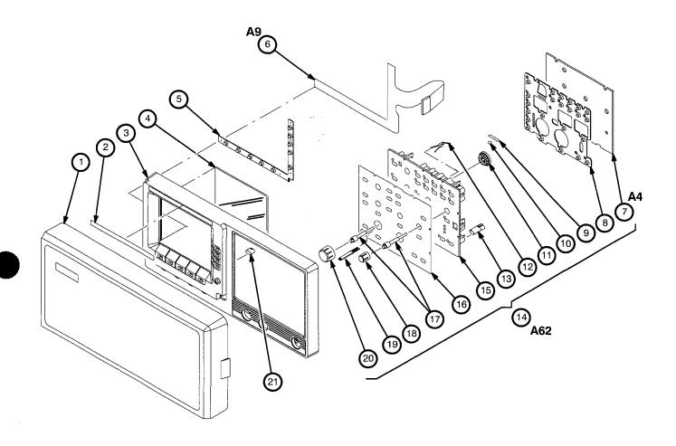
Figure 10-2: Front Panel Assembly
