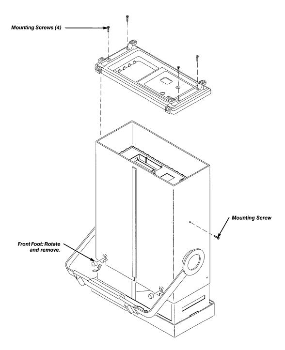
Figure 6-7: Rear Cover, Cabinet, and Feet Removal
