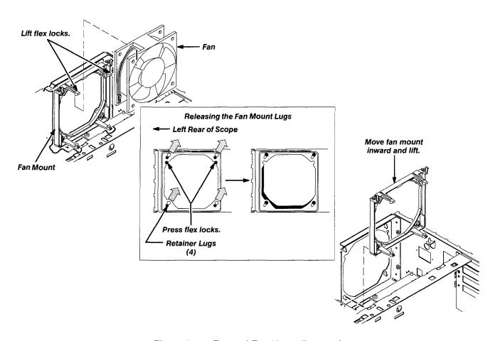
Figure 6-19: Fan and Fan Mount Removal
