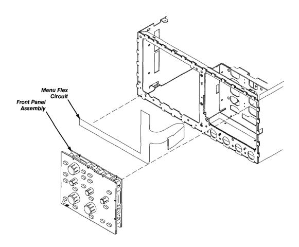
Figure 6-12: Menu Flex Circuit Board Removal
