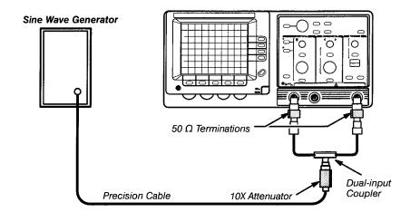
Figure 4-13: Trigger Sensitivity Test Setup Two
