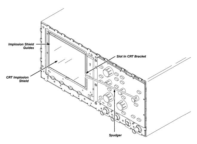
Figure 6-14: CRT Implosion Shield Removal
