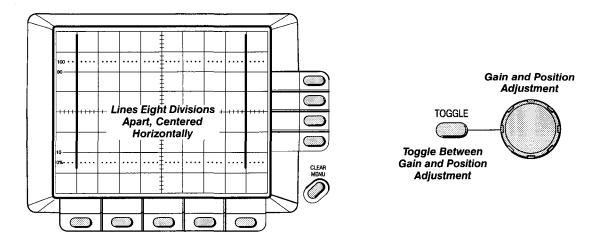
Figure 5-6: Horizontal Adjustments
