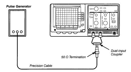
Figure 5-3: Low Frequency Output Compensation Calibration Setup
