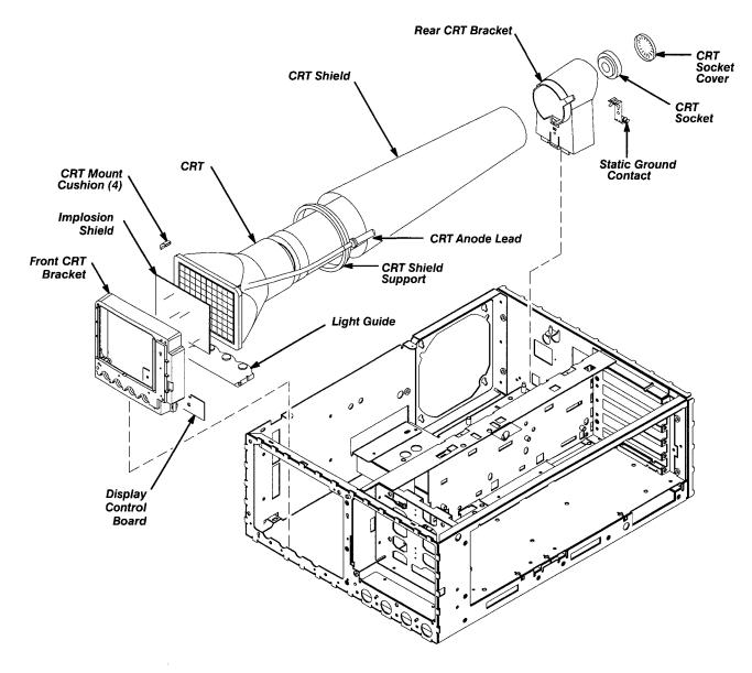
Figure 6-16: CRT Removal
