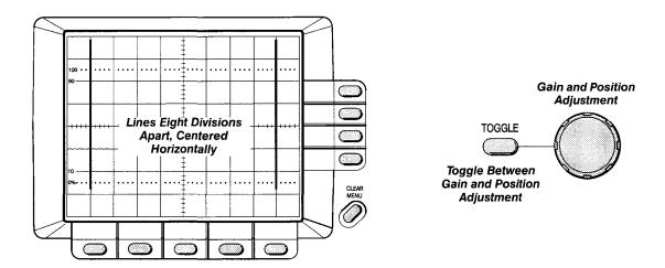
Figure 4-5: Horizontal Adjustments (Three)
