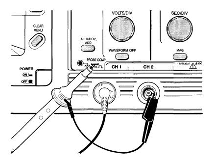
Figure 2-5: Connections for Compensating a Probe
