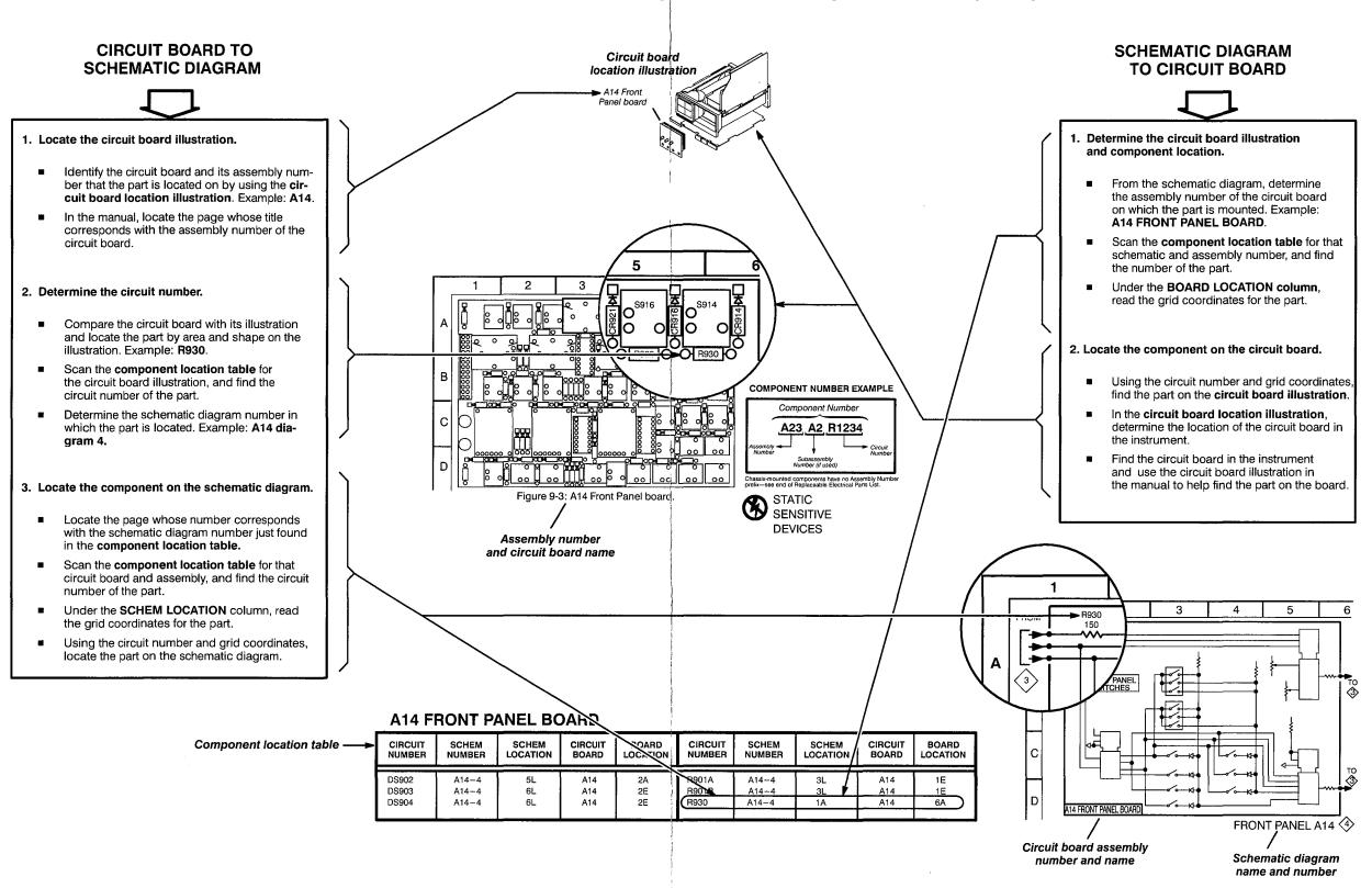
Figure 9-4: Locating Components on Circuit Board or Schematic Diagram
