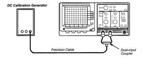
Figure 5-8: Factory Vertical Calibration Setup
