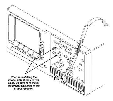
Figure 6-6: Knob and Shaft Removal
