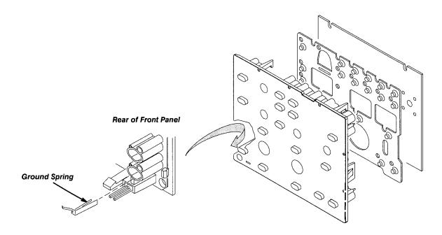
Figure 6-11: Front-Panel Ground Spring
