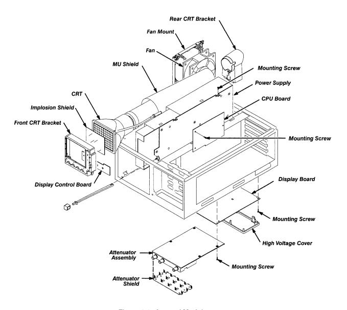
Figure 6-3: Internal Modules
