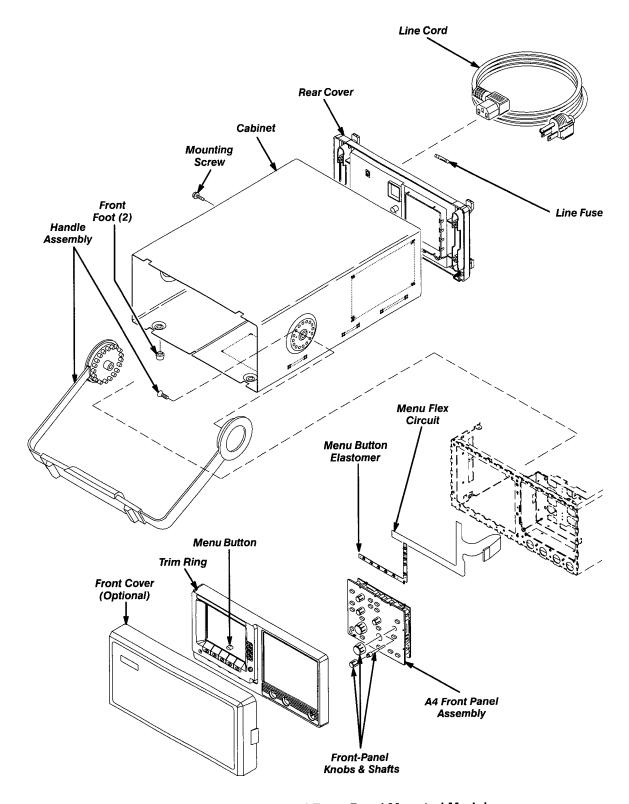
Figure 6-2: Cabinet and Front-Panel Mounted Modules
