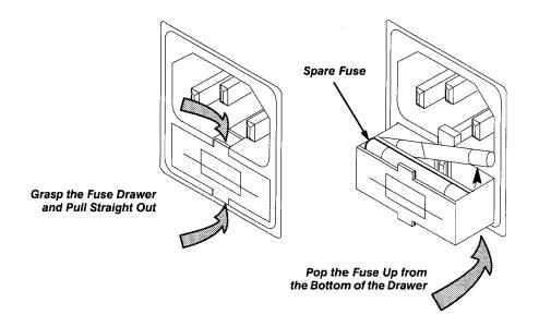
Figure 2-2: Fuse Compartment
