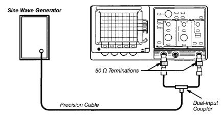
Figure 4-14: Trigger Sensitivity Test Setup Three
