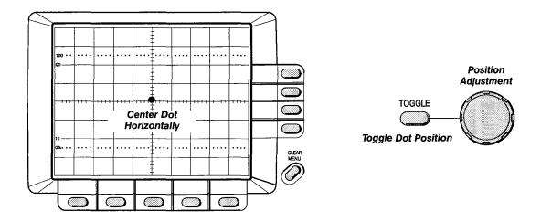
Figure 4-4: Horizontal Adjustments (Two)
