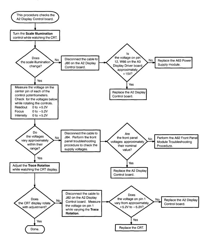
Figure 6-24: A2 Display Control Board Troubleshooting Procedure
