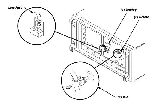
Figure 6-5: Line Fuse and Line Cord Removal
