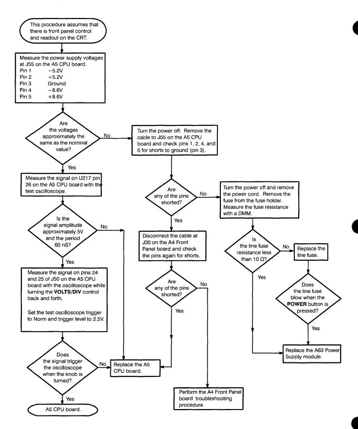
Figure 6-20: A5 CPU Board Troubleshooting Procedure
