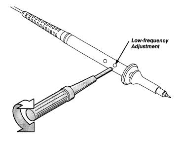
Figure 2-7: Location of Probe Head Adjustment
