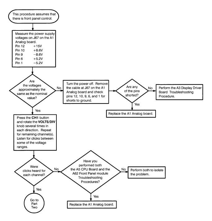
Figure 6-21: A1 Analog Board Troubleshooting Procedure
