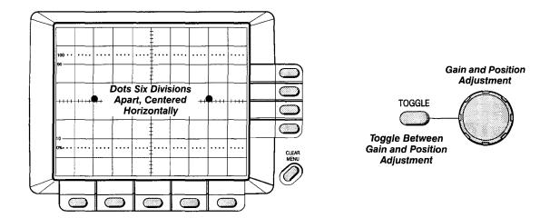
Figure 5-10: Vertical Adjustments
