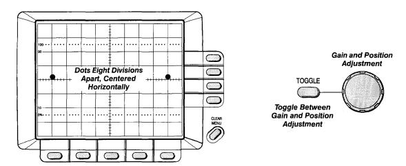
Figure 5-4: Horizontal Adjustments
