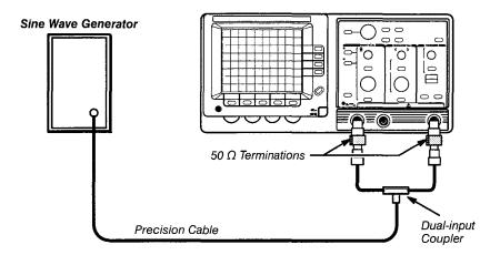
Figure 4-12: Trigger Sensitivity Test Setup One
