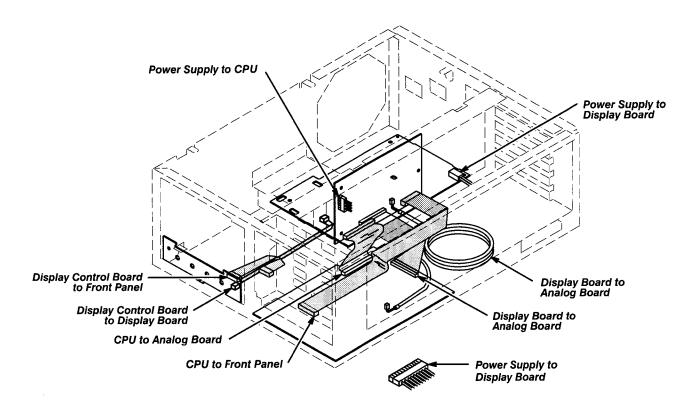
Figure 6-4: Cables and Cable Routing
