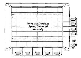
Figure 5-11: Adjusting Vertical Gain and Centering
