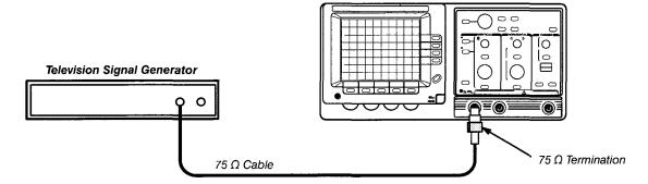
Figure 4-16: Video Trigger Test Setup
