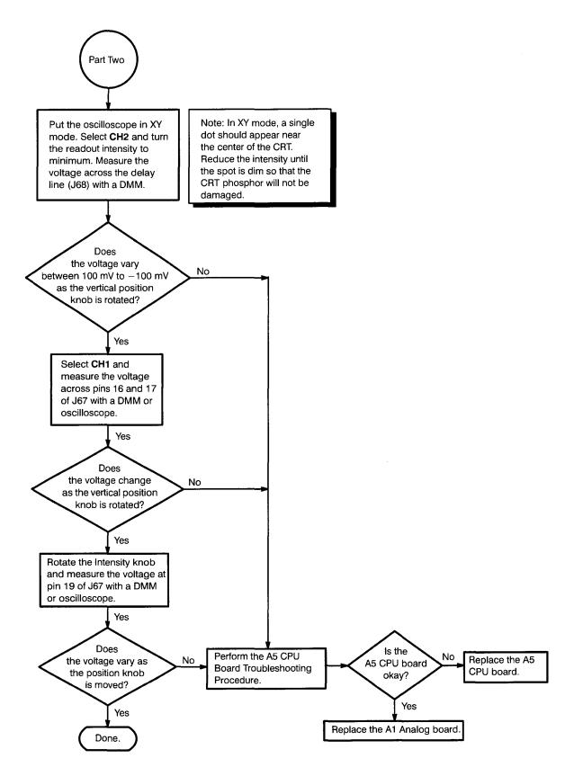
Figure 6-21: A1 Analog Board Troubleshooting Procedure (Cont.)
