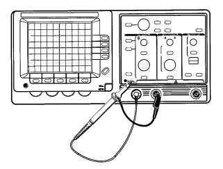
Figure 4-2: Test Hookup for Functional Tests
