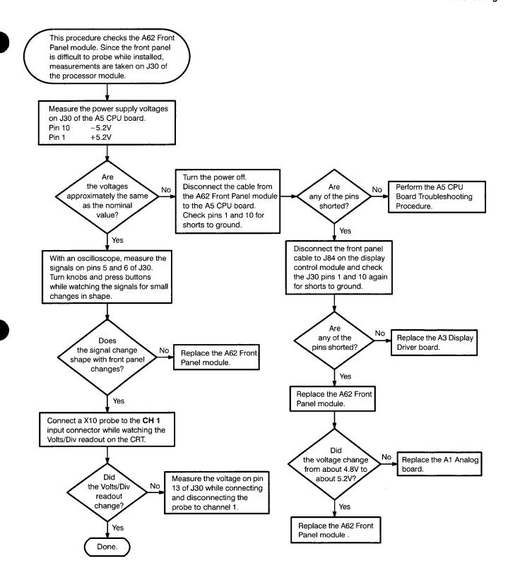
Figure 6-23: A62 Front Panel module Troubleshooting Procedure
