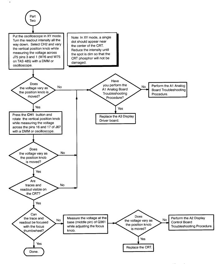
Figure 6-22: A3 Display Driver Board Troubleshooting Procedure (Cont.)
