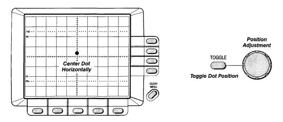
Figure 5-5: Horizontal Adjustments
