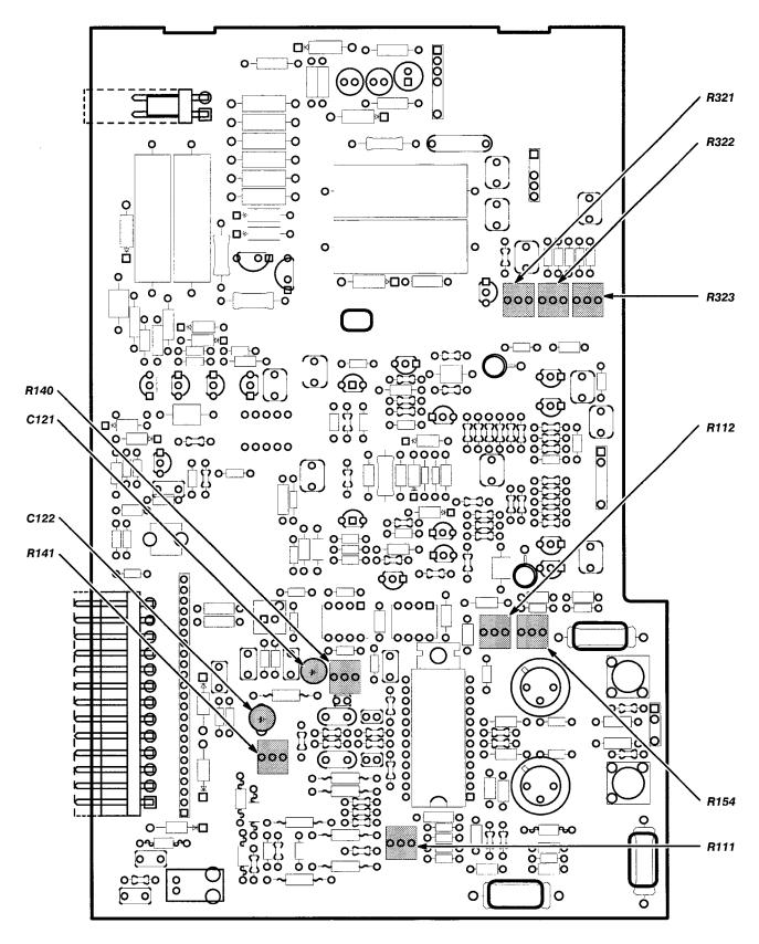
Figure 5-14: Display Driver Board Adjustment Locations
