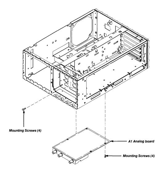
Figure 6-13: A1 Analog Board Removal
