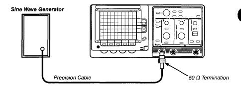
Figure 4-8: Bandwidth Test Setup
