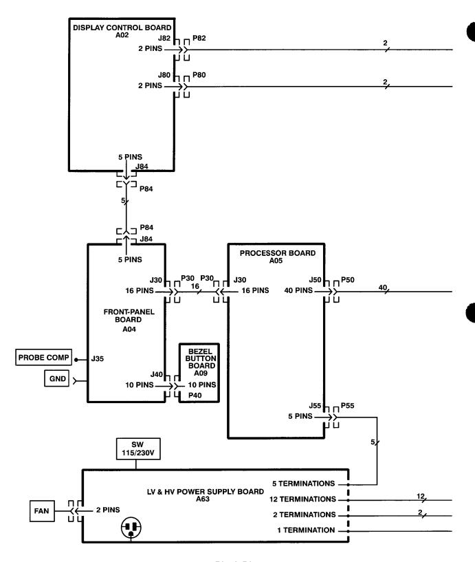
Figure 3-1: Block Diagram
