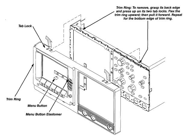
Figure 6-8: Trim Ring and Menu Buttons Removal
