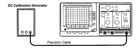
Figure 5-9: External Trigger Calibration Setup
