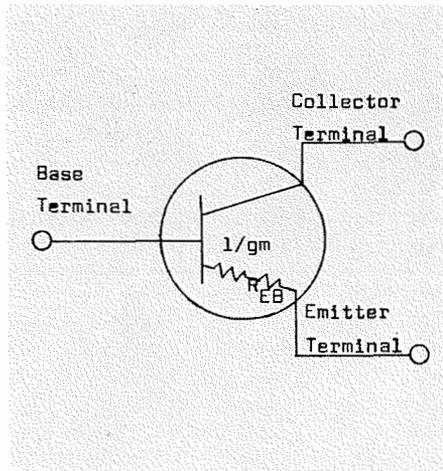
Figure 2 — Schematic equivalent of the emitter circuit of a transistor.  $1/gm$  is the dynamic resistance of the junction due to carrier action and  $R_{EB}$  is the DC resistance in the leads and ohmic contacts of the leads within the transistor case.
