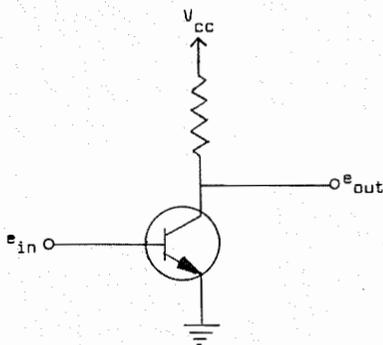
Figure 4 — Amplifier used as an example of the application of transresistance compared to h-parameters. The DC operating point is assumed to be set at  $I_e = 5 \text{ ma}$ ;  $V_{ce} = 2.5 \text{ v}$ . The transistor is a 2N2475.
