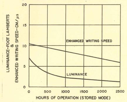
The brightness and contrast ratio are measured at the operating point and the writing speed is measured at 60  $\mu$ A.
