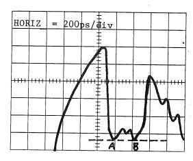
The following is an S-4, Inline TD waveform illustrating the 0% and 100% amplitude points and the 10% and 90% risetime points.
