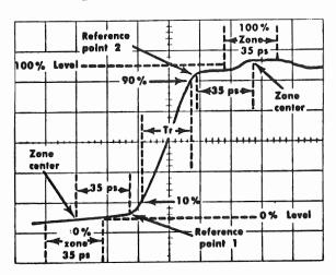
Two reference points are chosen at the points where the slope is at its maximum rate of change. The 0% and 100% levels are the average amplitude within the zones which are one t<sub>r</sub> (the specified combined risetime of the TYPE S-4 and TYPE S-50, 35ps) in width. The 0% zone is centered 1 t<sub>r</sub> before the first reference point and the 100% zone is centered 1 t<sub>r</sub> after the second reference point.
