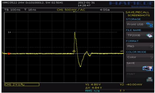
TP235: measure at 50% amplitude 2V/div, 340nS pulse width (delta 30 nS)
