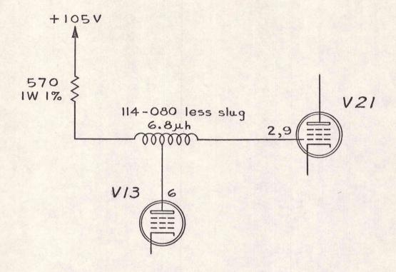
This assembly simulates one section of the delay line and makes possible normal compensation of the distributed amplifier. The vertical amplifier may be checked for risetime and bandwidth with this network installed. It makes possible delay line adjustment without further vertical distributed amplifier tuning. (It is possible to tune the distributed amp without the "T" coil but with poorer results.)
