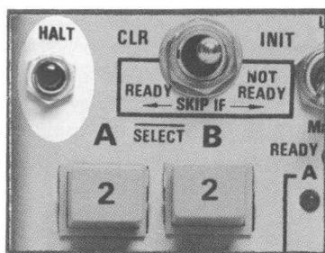
This dual purpose pushbutton switch can be used (1) to produce a HALT instruction for a program that is being stored in the memory, or (2) when the M/P Card is in a Programmed mode, it can be used to stop an automatic sequence. When this switch is used to stop a program process, the program can be started again by pressing either the DI or DO pushbuttons.
