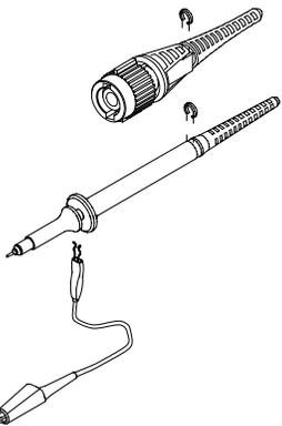
Marker rings — Attach the matching colored rings onto the probe cable and tip as shown.
