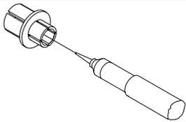
BNC-to-probe tip adapter — To install the adapter, push the wide end firmly into a BNC connector. Then insert the probe tip firmly into the adapter.
