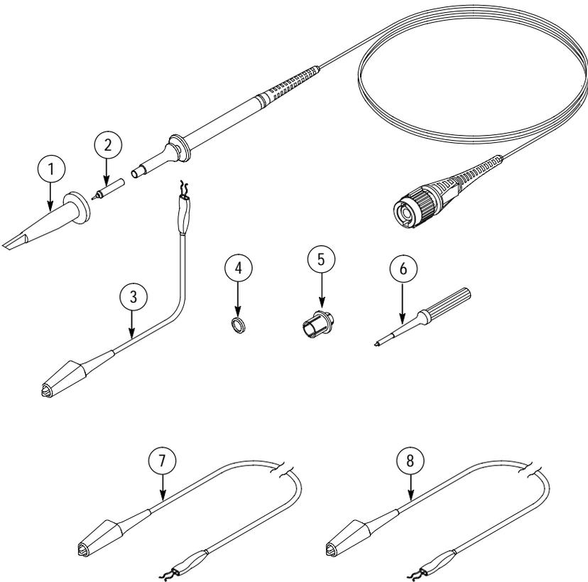
Figure 3: P6119B Replaceable Parts
