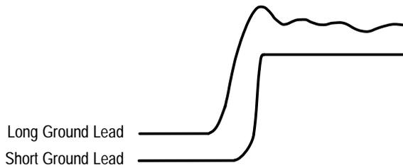
To see the best signal, use the shortest possible ground lead and signal path.
