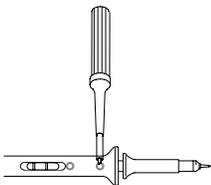
Adjustment tool — Use the adjustment tool for probe compensation adjustments.
