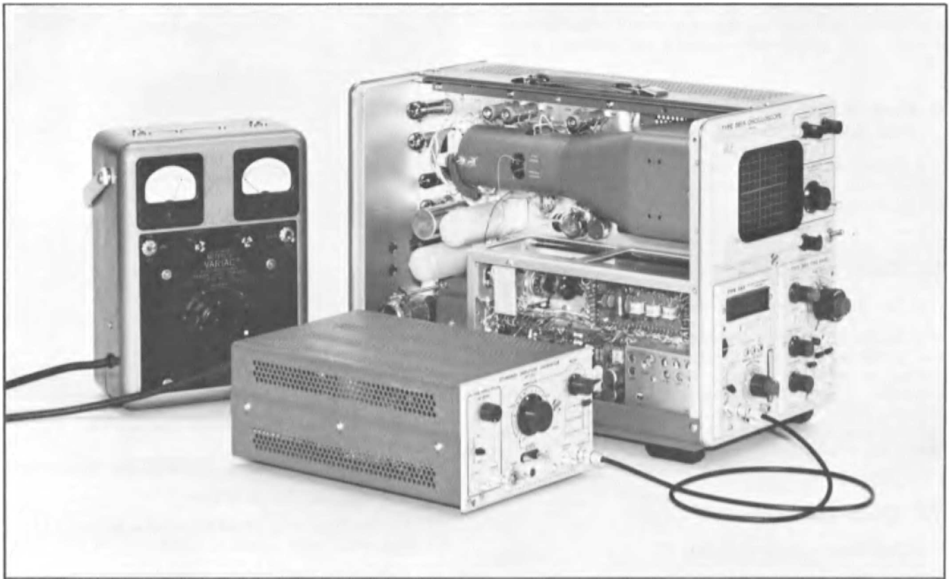
Fig. 6-7. Test setup for adjusting Vertical Amplifier gain.
