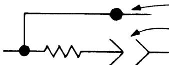
Connection soldered to circuit board.
