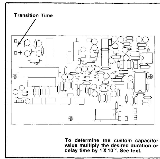
Fig. 1-3. Location for transition custom timing capacitor.
