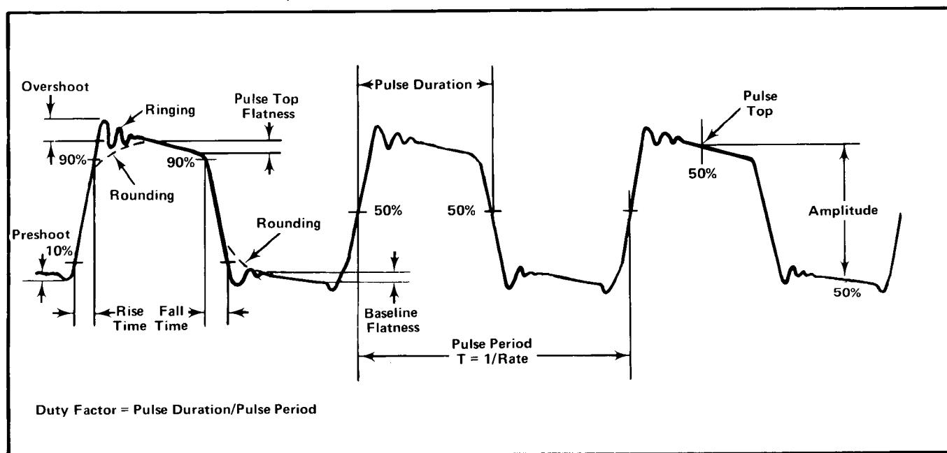
Fig. 1-5. Pulse characteristics.
