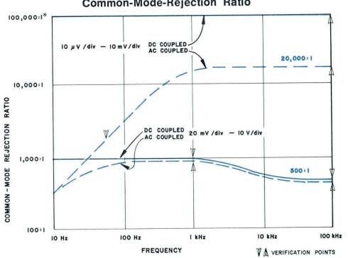
\*With up to 20-V peak-to-peak sinewave. CMRR is not specified when display is 0.1 div or less from DC to 1 kHz, or 0.2 div or less from 1 kHz to 100 kHz.
