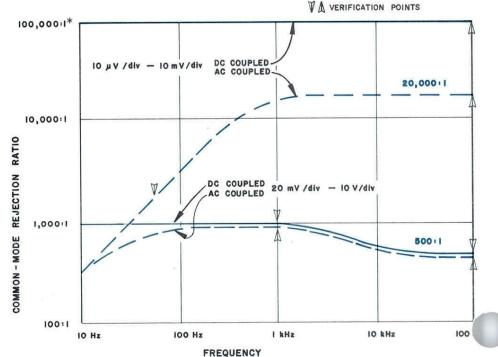
\*With up to 20-V peak-to-peak sinewave. CMRR is not specified when display is 0.1 div or less from DC to 1 kHz, or 0.2 div or less from 1 kHz to 100 kHz.
