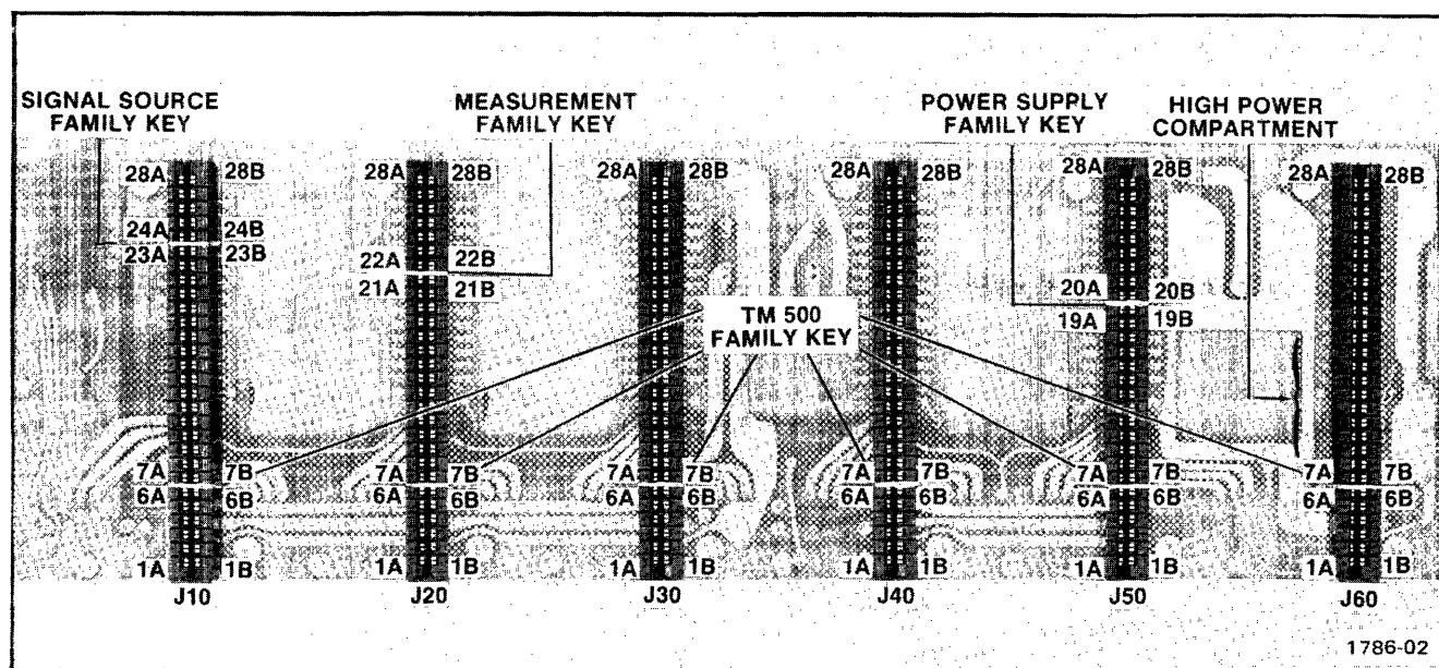
Fig. 2-1. Keying assignments for family functions. One of many possible sequence combinations.
