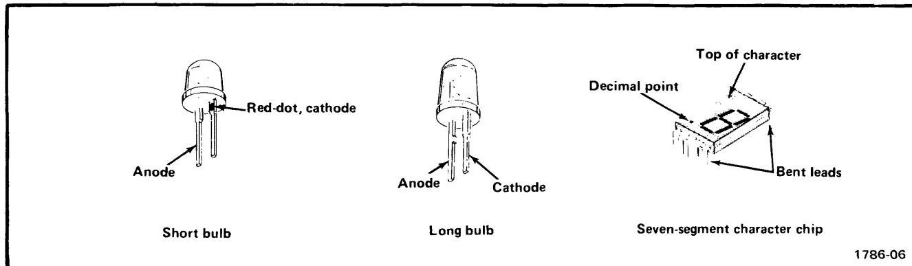
Fig. 3-2. Light-emitting diode (LED) lead orientation illustration.
