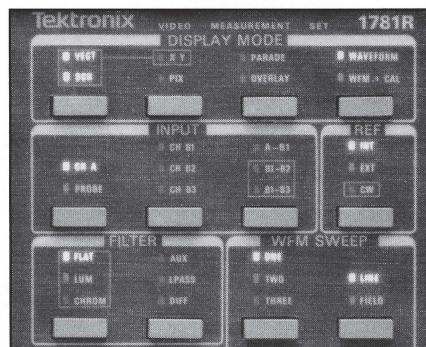
Multiple inputs and parade display mode facilitates component signal measurements.
