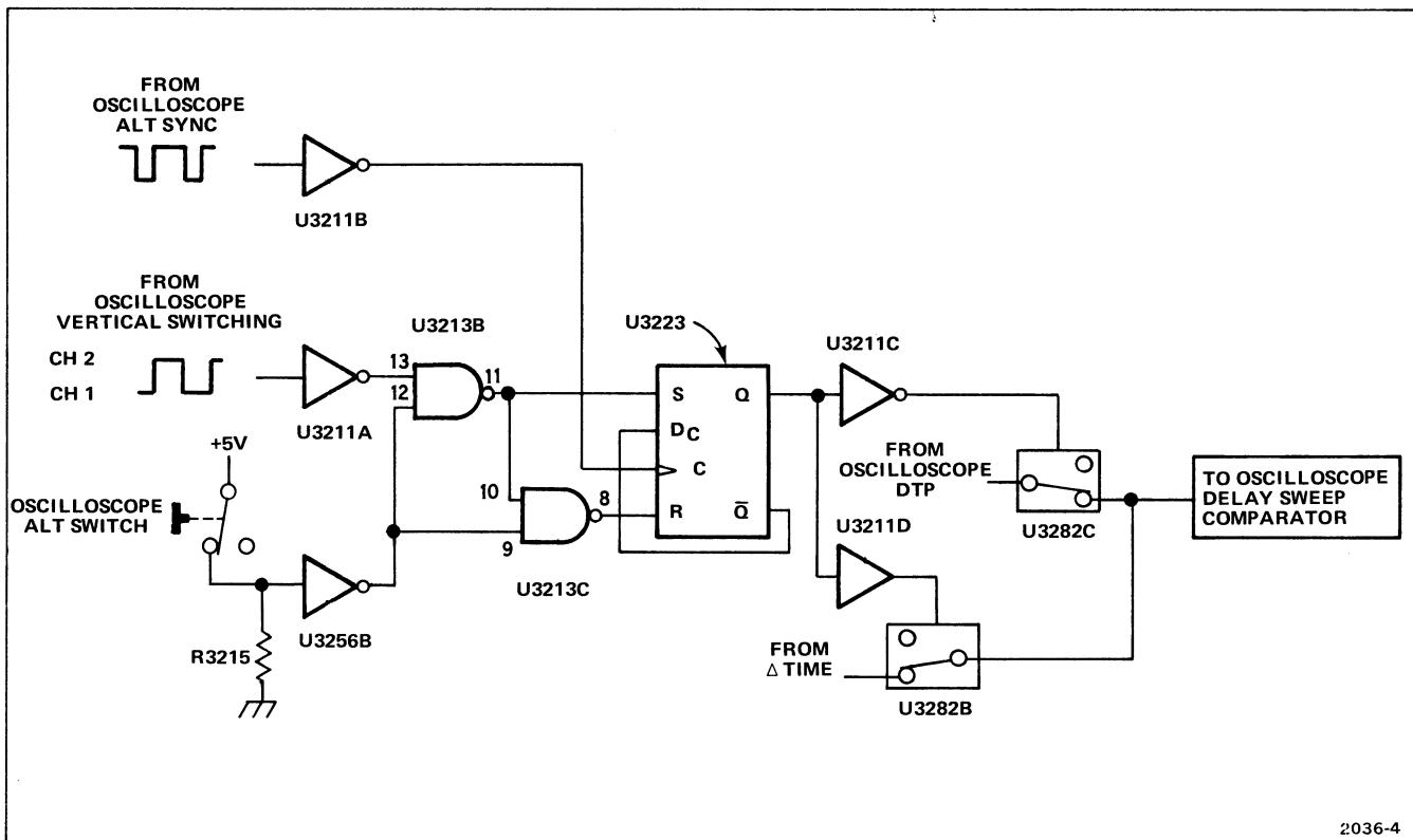
Figure 4-7. Simplified diagram of the Delay Pickoff Selector Logic.
