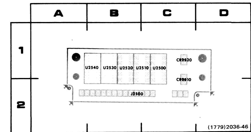
Fig. 9-5. A2 Readout board component locations.
