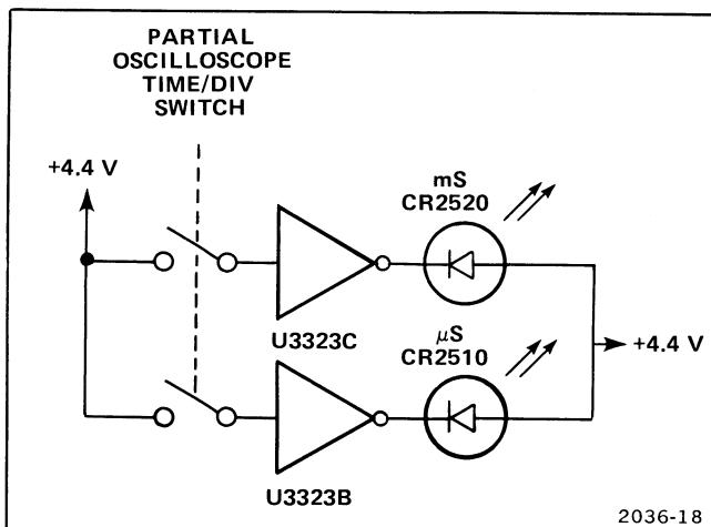
Figure 4-20. Simplified diagram of ms and  $\mu$ s Logic when in the TIME function.
