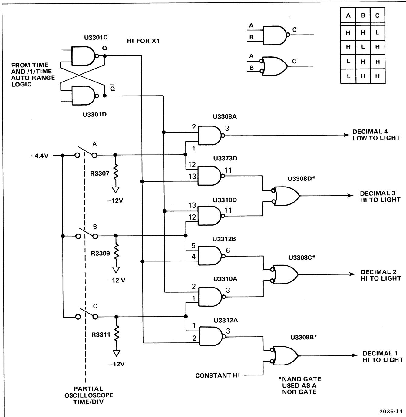
Figure 4-18. Simplified diagram of TIME and 1/TIME Decimal Logic.
