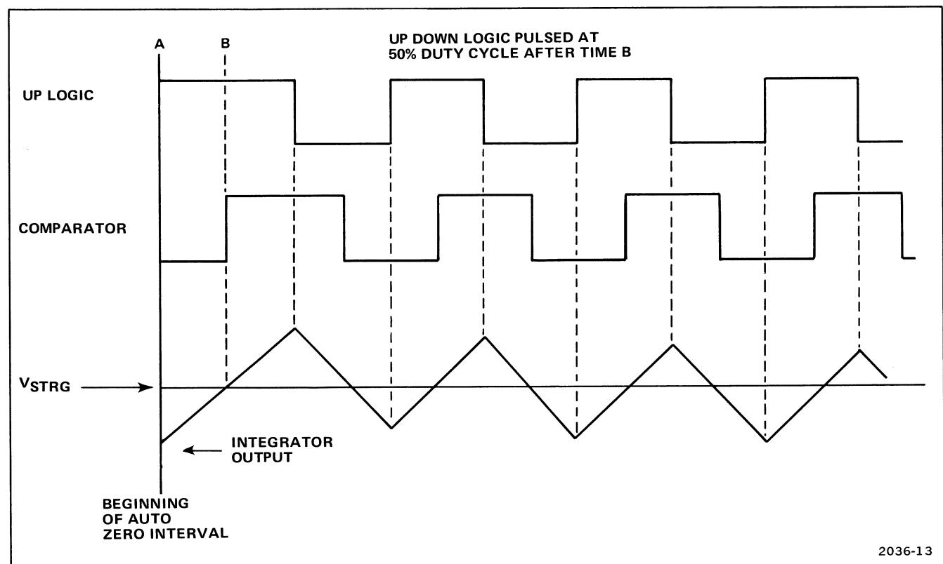
Figure 4-12. Auto Zero Interval timing.
