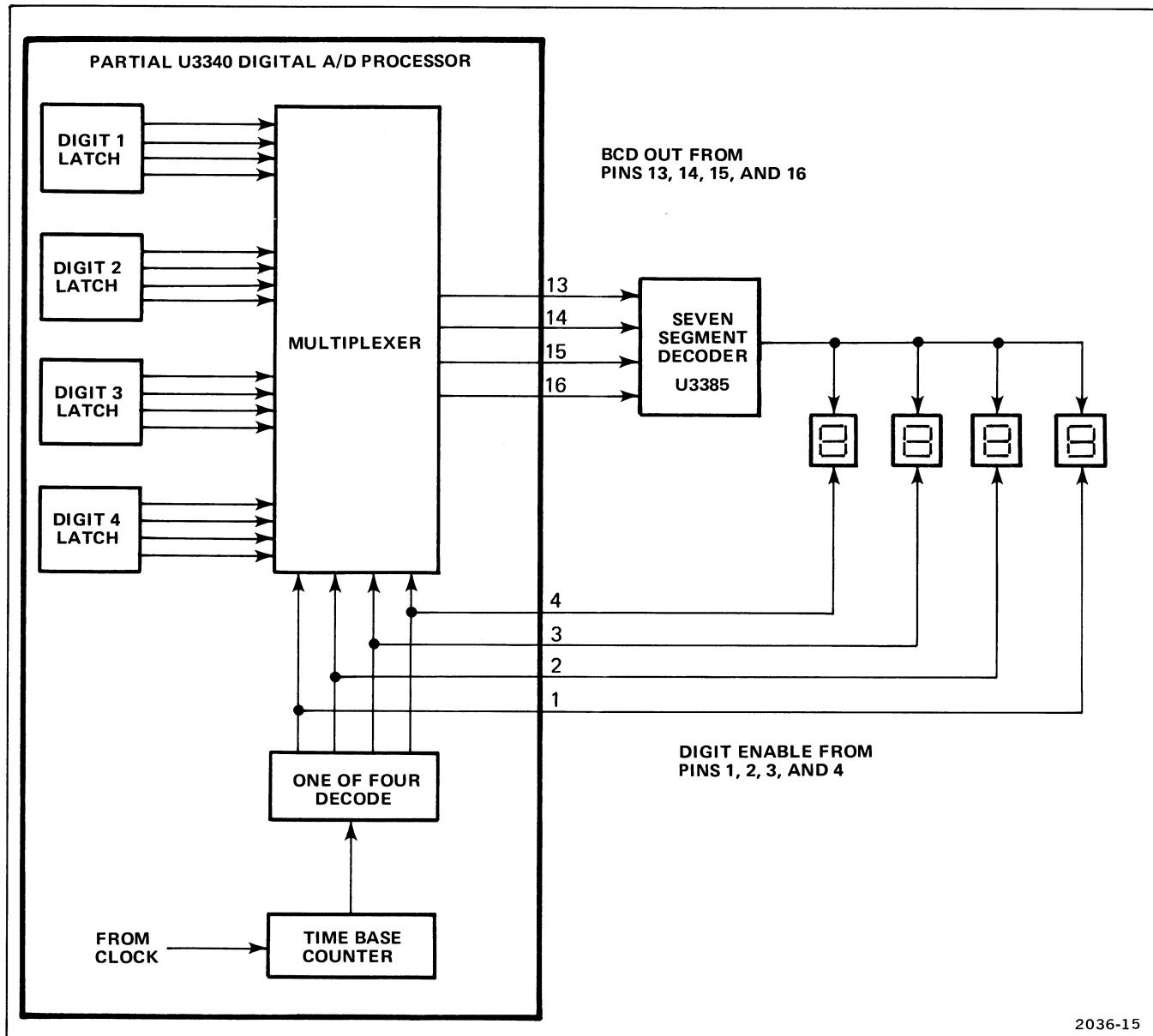
Figure 4-17. Simplified diagram of the Readout Logic.
