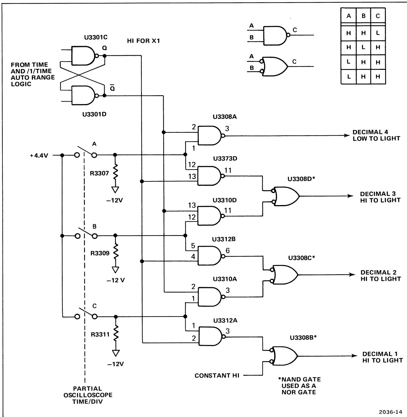
Figure 4-18. Simplified diagram of TIME and 1/TIME Decimal Logic.
