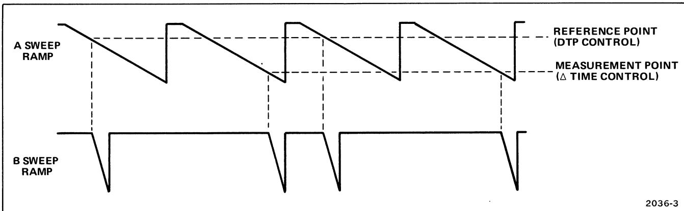
Figure 4-8. Delay Pickoff Selector Logic selects which control determines the beginning of B Sweep.
