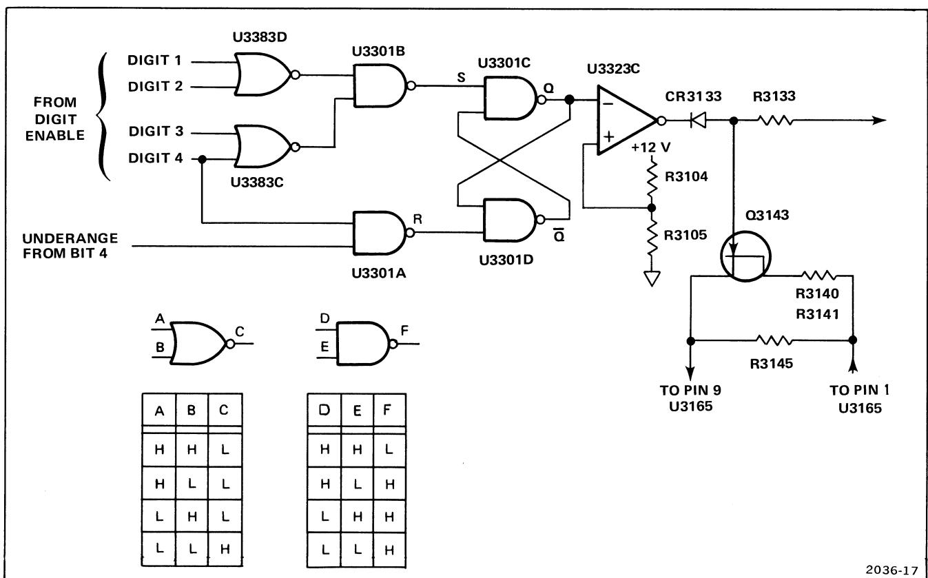
Figure 4-21. Simplified diagram of TIME and 1/TIME Autorange Logic.
