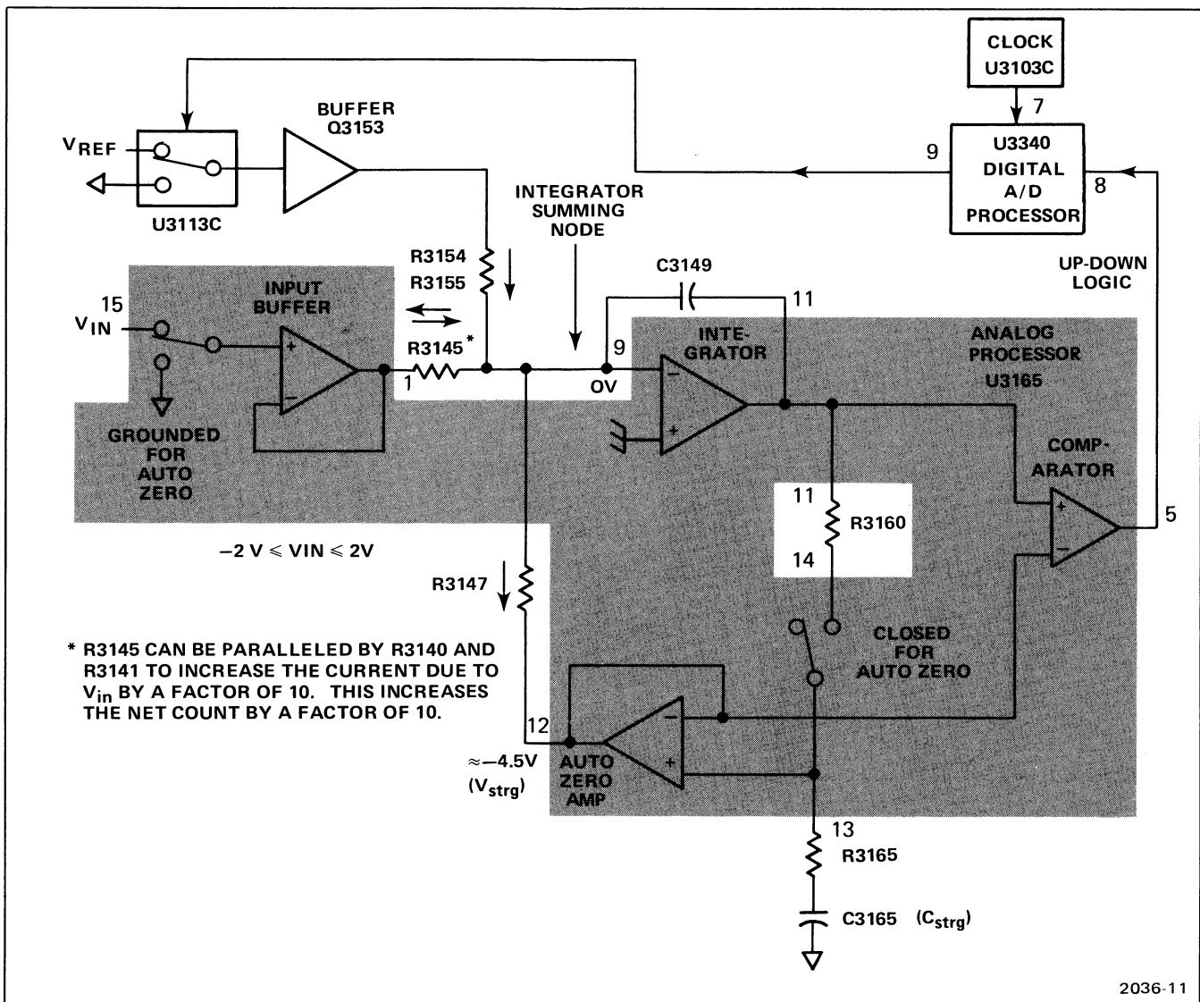
Figure 4-13. Simplified diagram of the Analog-to-Digital Converter.
