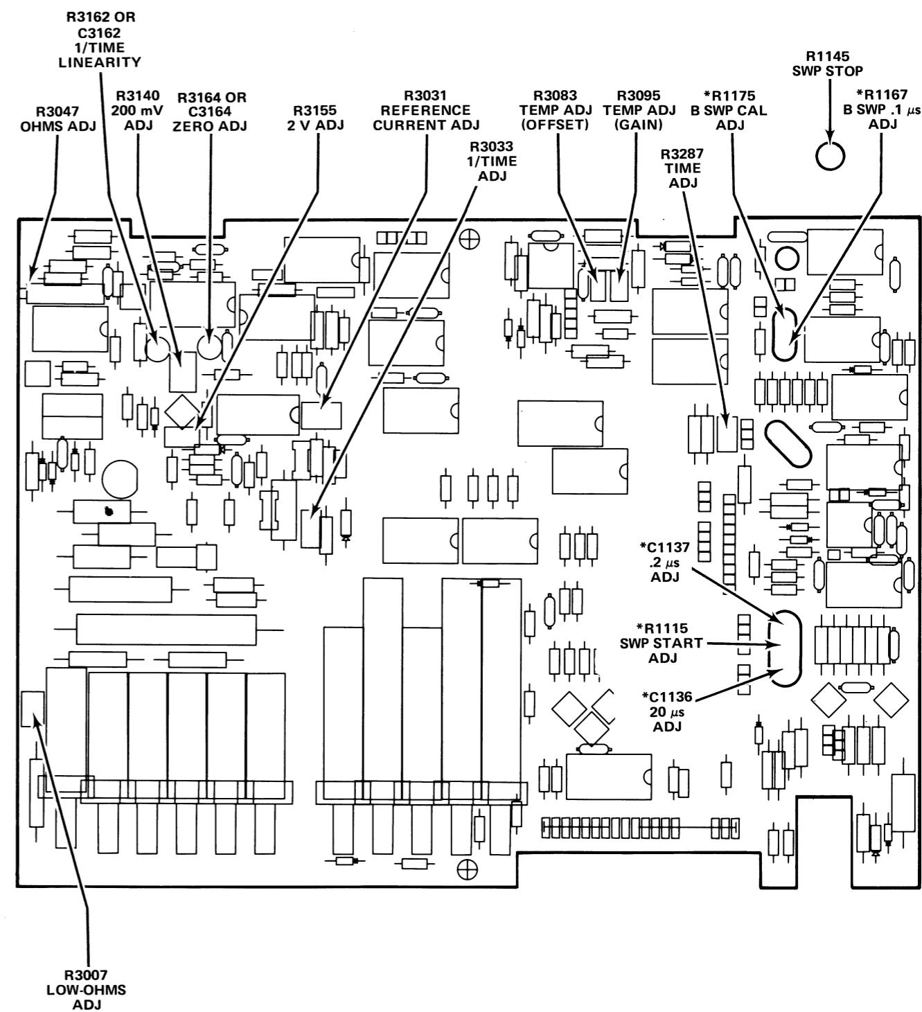
\*PARTS MOUNTED ON OSCILLOSCOPE TIMING BOARD,
