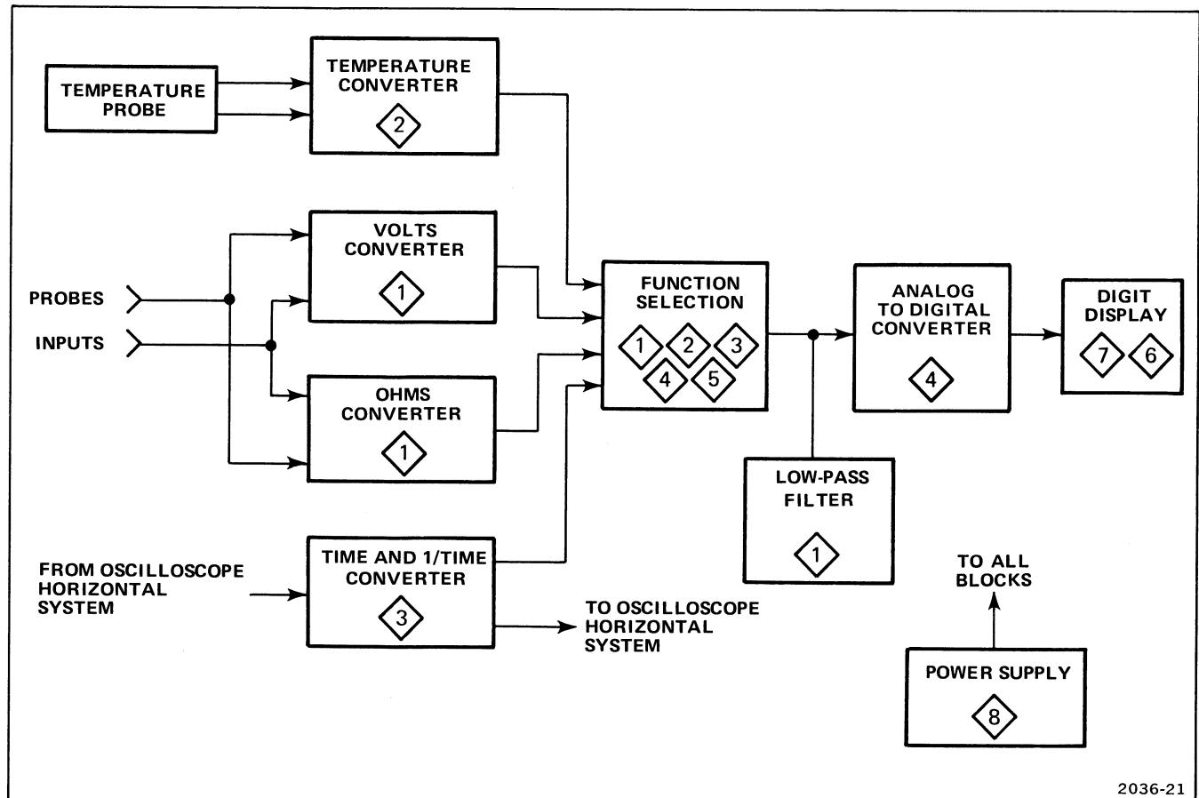
Figure 4-1. Simplified block diagram of the DM44.
