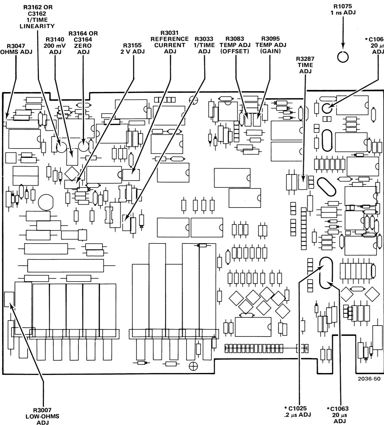
FIG. 9-15A AND FIG. 9-15B SHOW DM44 ADJUSTMENTS AND OSCILLOSCOPE ADJUSTMENTS LOCATED UNDER THE DM44 MAIN BOARD. FOR OTHER ADJUSTMENTS, SEE THE OSCILLOSCOPE SERVICE OR INSTRUCTION MANUAL.
