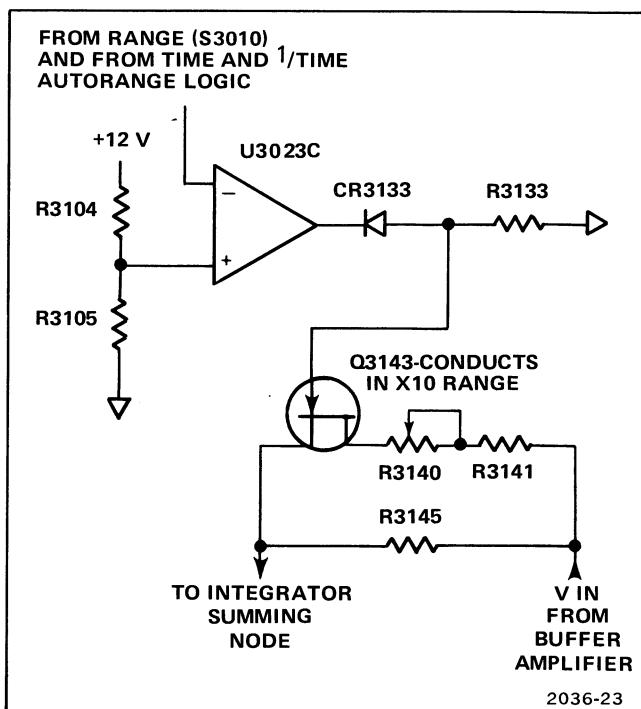
Figure 4-15. Simplified diagram of the Integrator Gain Switching circuit.
