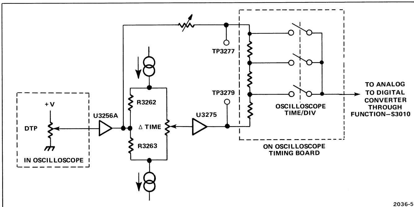
Figure 4-6. Obtaining a voltage proportional to the time interval being measured.
