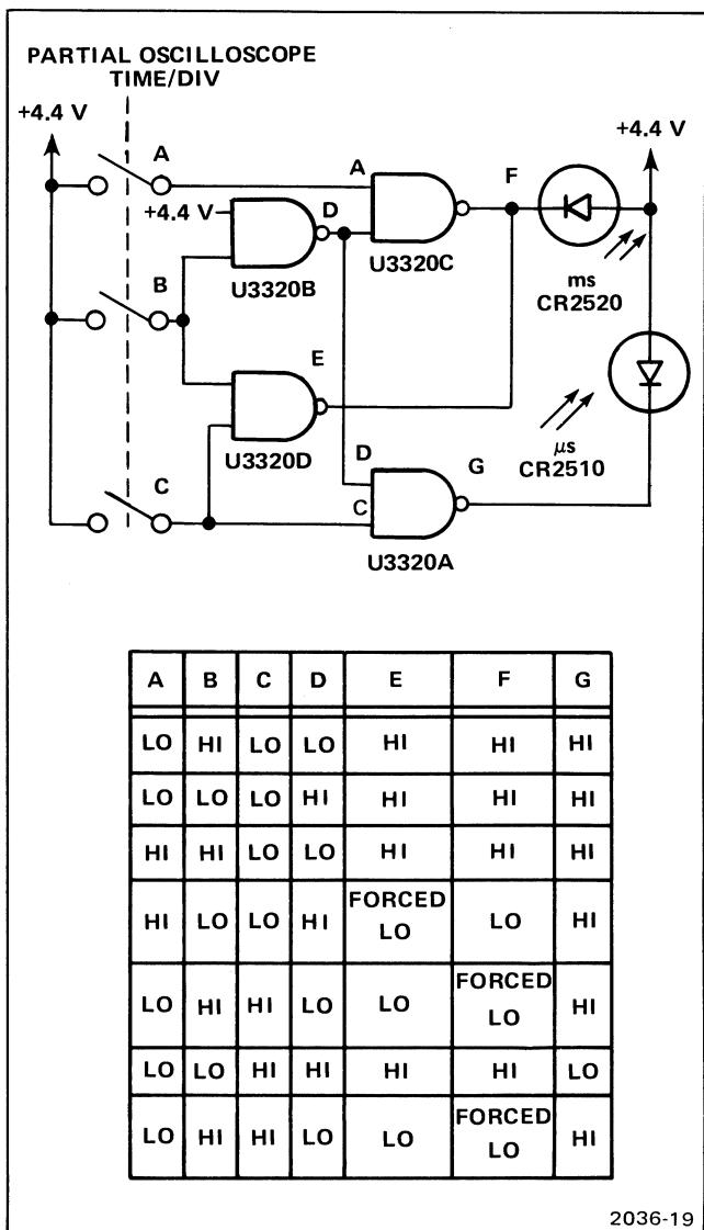
Figure 4-19. Simplified diagram of ms and  $\mu$ s Logic when in the 1/TIME function.
