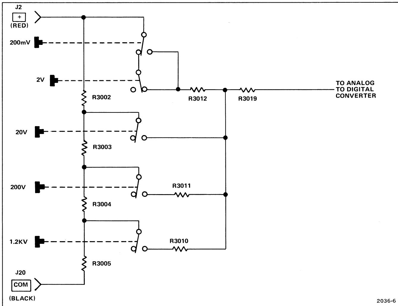
Figure 4-3. Simplified diagram of the VOLTS Converter.
