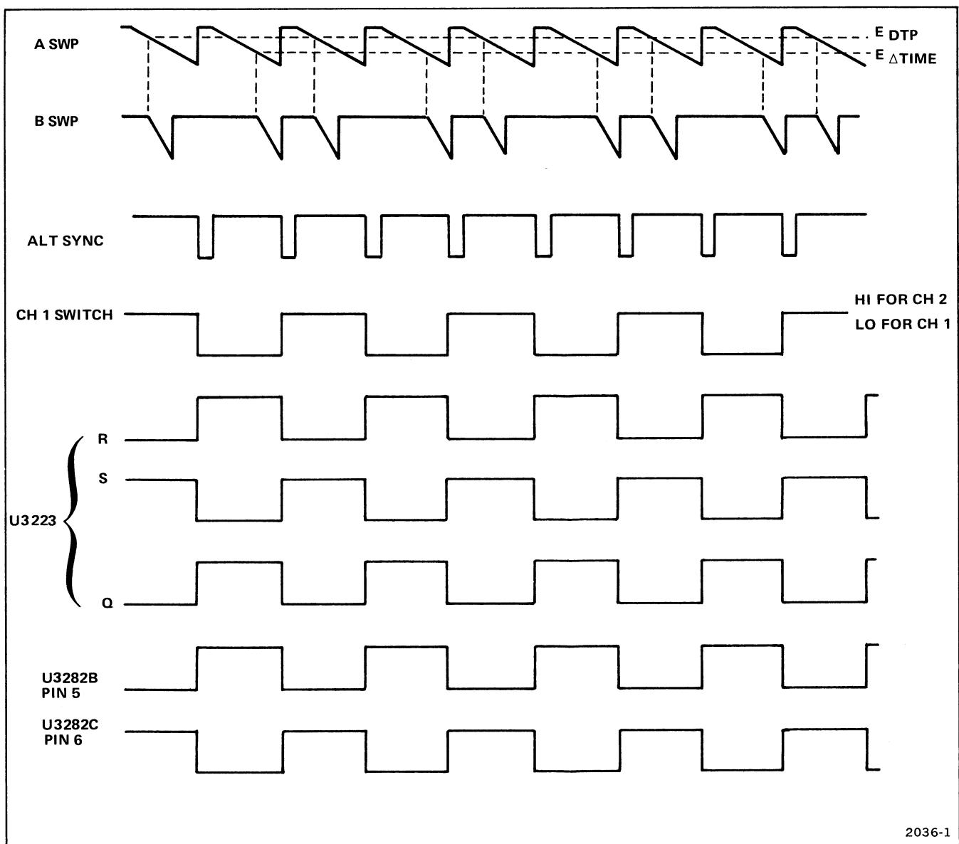
Figure 4-9. Timing diagram of Delay Pickoff Selector Logic signals generated in the ALT vertical mode.
