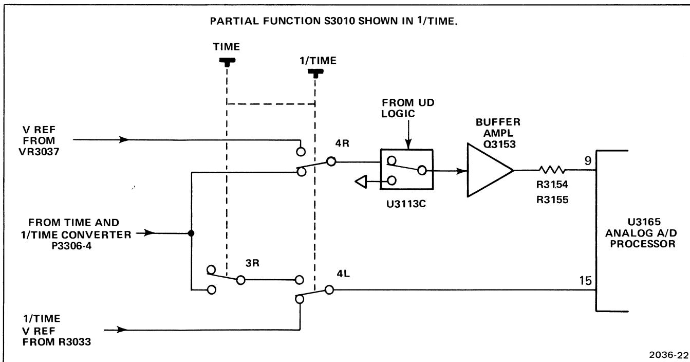
Figure 4-10. 1/TIME Function switching.
