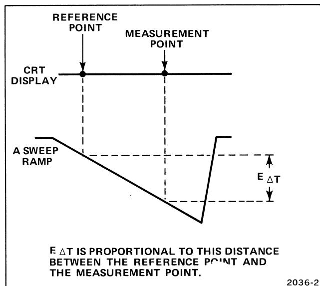
Figure 4-5. Basic function of the TIME and 1/TIME Cc
