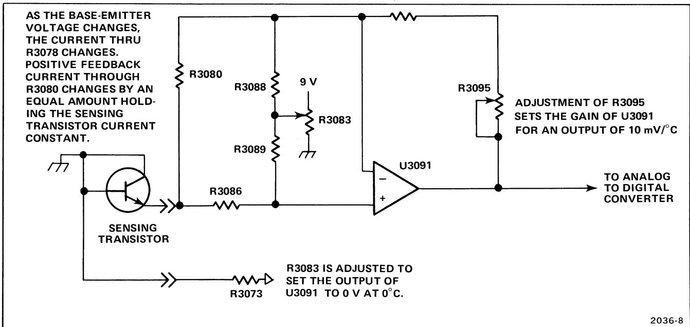
Figure 4-2. Simplified diagram of the Temperature Converter.
