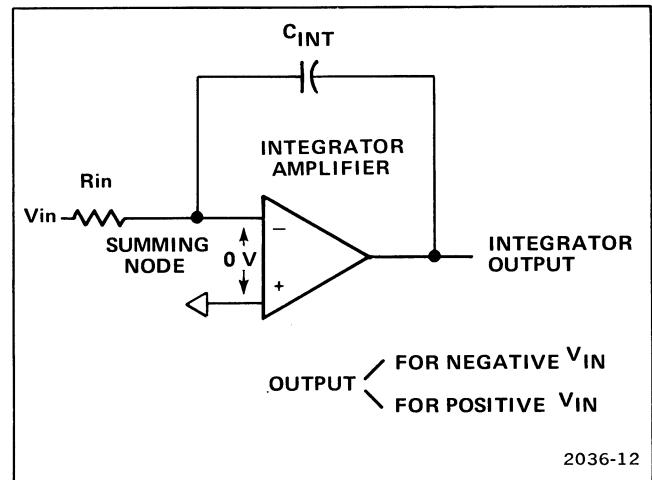
Figure 4-11. Simplified diagram of a basic integrator.
