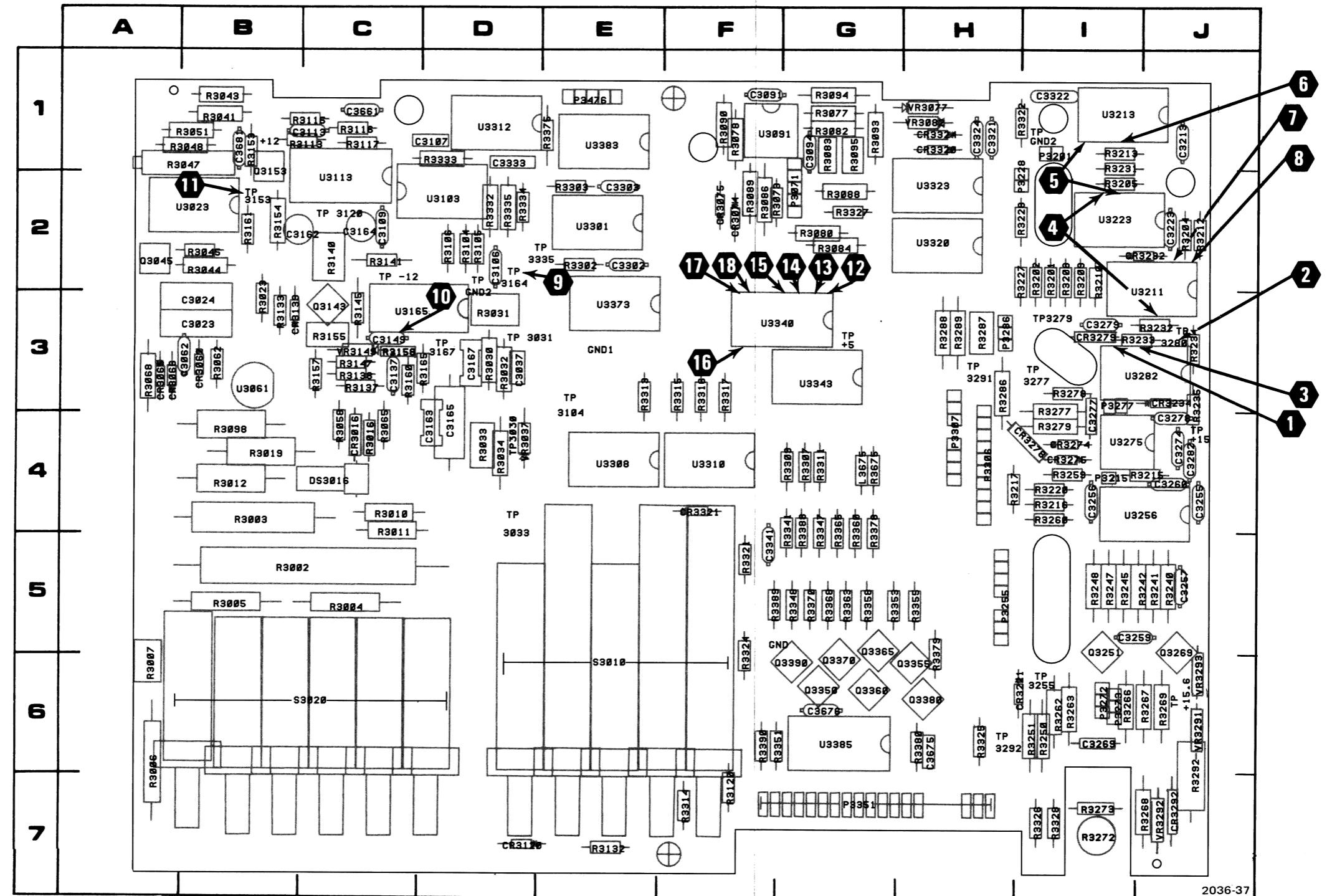
Fig. 9-3. A1 Main board component locations (SN B010100-B019999).
