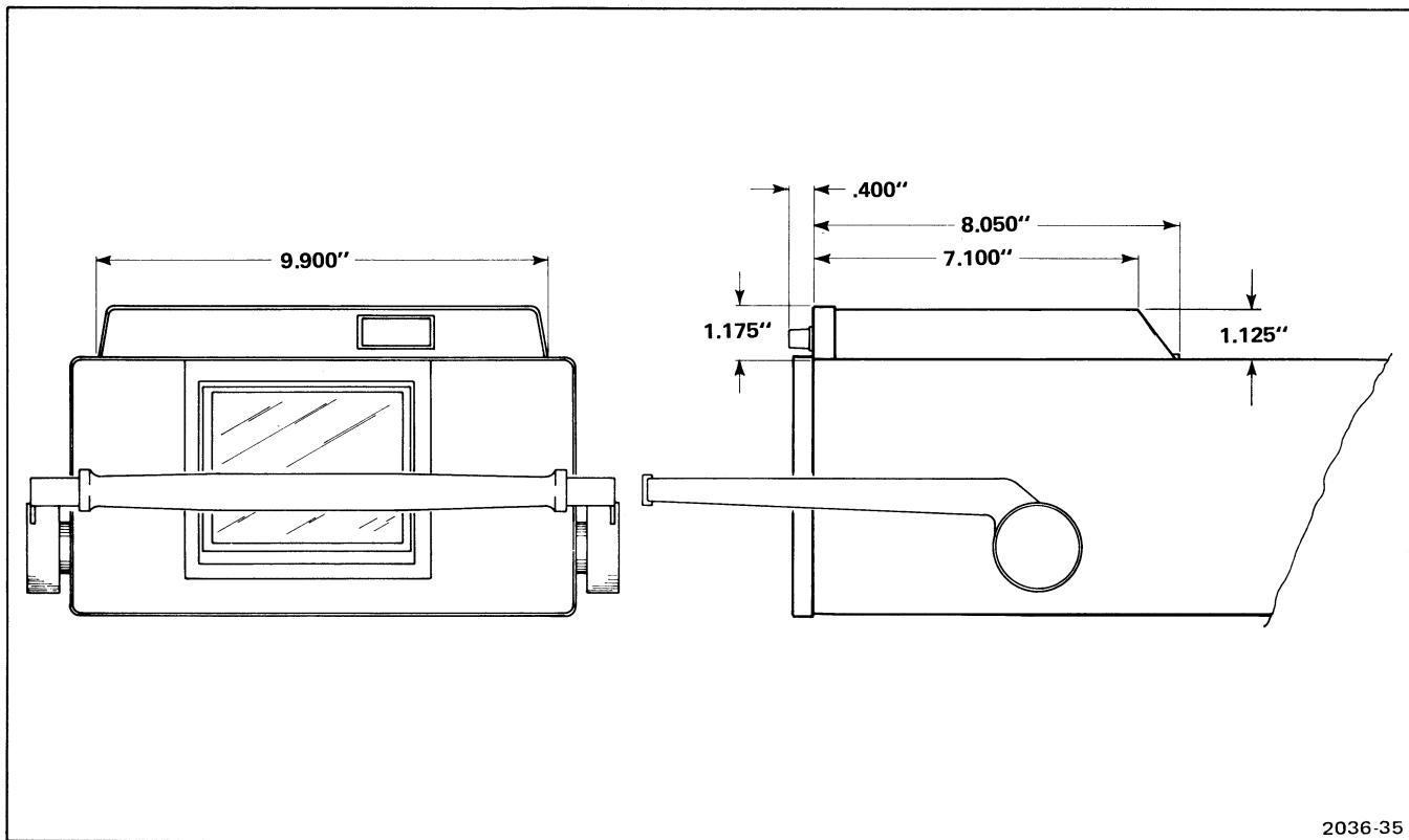
Figure 1-1. DM44 dimensional drawing.
