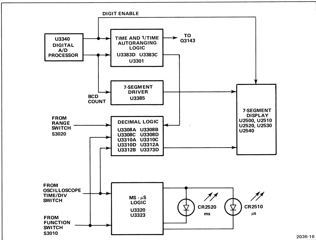
Figure 4-16. Block diagram of the Readout Display and associated circuitry.
