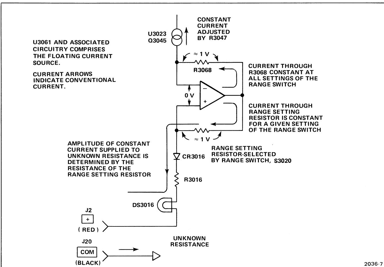
Figure 4-4. Simplified diagram of the OHMS Converter.
