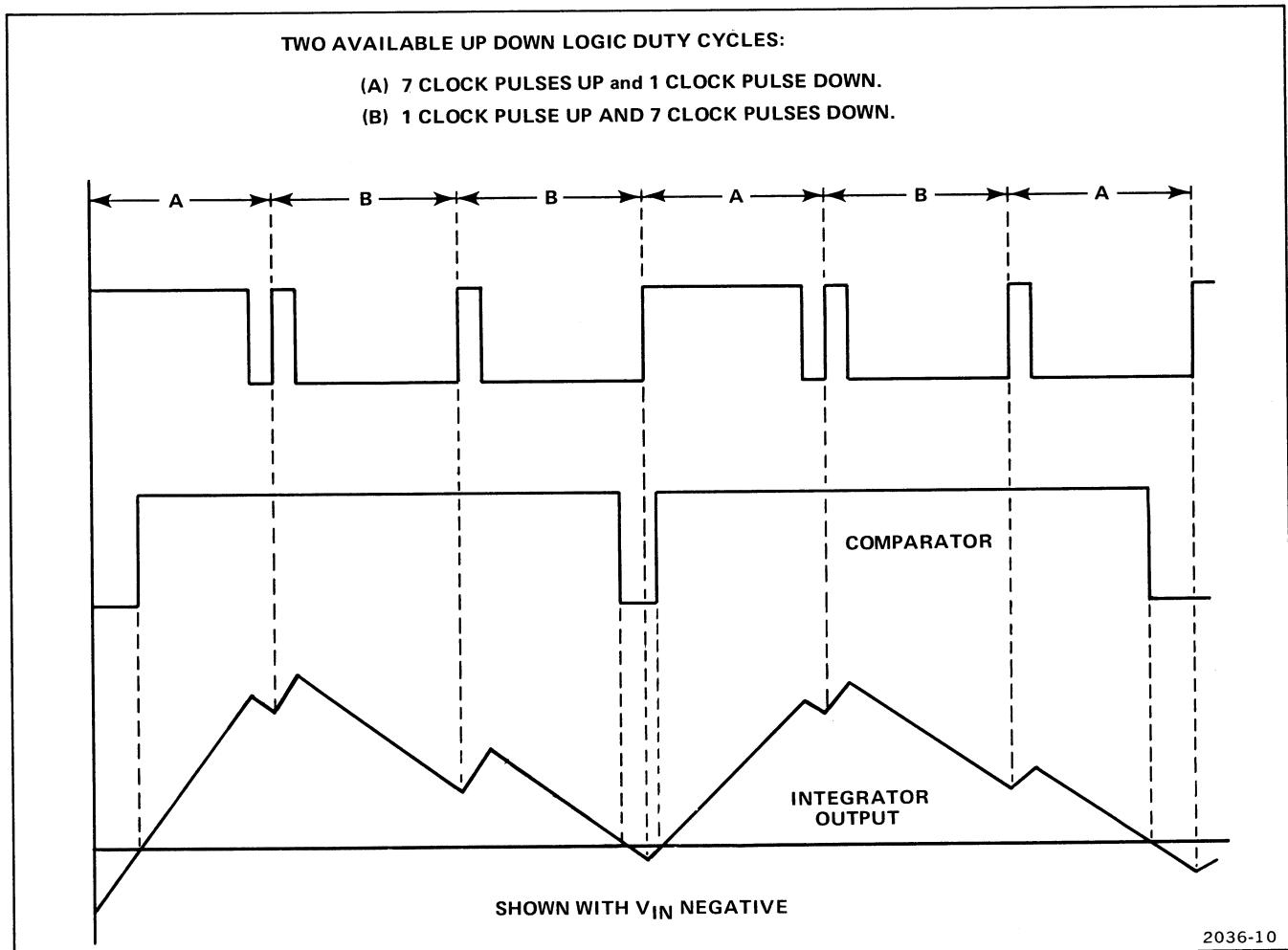
Figure 4-14. Measure interval timing with negative  $V_{\text{in}}$ .
