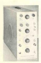
Type 112 DC-Coupled Differential Amplifier provides a voltage gain of 0.5 to 5000, continuously variable. Frequency response is dc to 2 mc for gains of 166 or less, and dc to 1 mc for gains of 166 to 5000. Output voltage is 150 v at high impedance, 75 v at 8000 ohms. Calibrator has range of 5 mv
