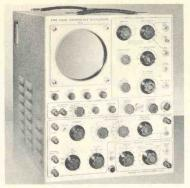
**Type 524AD Television Oscilloscope** is designed for TV transmitter and studio use for both monochrome and color, and has the following features: 0.1-μsec/cm to 0.01-sec/cm sweeps, with zero to 25 milliseconds delay, a line at a time, on all sweeps; 3-x and 10-x magnification, accurate within 2% except at sweep times less than 0.1 μsec/cm; field selector for switching to either field of a frame; builtin sync separator; 60-cycle sine-wave sweep with amplitude and phase control;
