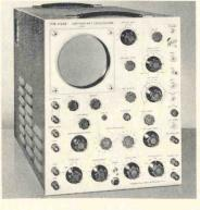
Type 514AD Oscilloscope features: 6-cm undistorted vertical deflection; variable-duty-cycle calibrator, dc-coupled unblanking. Vertical-amplifier passband dc to 10 mc at 0.3-v/cm to 100-v/cm sensitivity, 2 cycles to 10 mc at 0.03-v/cm to 100-v/cm sensitivity, risetime 0.04 µsec, 0.25-µsec signal delay. Sweep range 0.1 µsec/cm to 0.01 sec/cm; magnifier, 5-x, except at sweep times less than 0.1 µsec/cm. Square-wave calibrator variable from 0 to 50 volts, full-scale calibrations accu-
