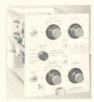
**Type 53C Dual-Trace Unit** — two identical amplifier channels, each with dc to 8.5 mc passband, 0.04-μsec risetime with Types 531 and 535...dc to 5 mc, 0.07-μsec risetime with Type 532. Sensitivity 0.05 v/cm to 50 v/cm continuously variable with 9 calibrated steps from 0.05 v/cm to 20 v/cm. Electronic switching triggered by sweep, or free running at about 100 kc. Weight 5½ lbs. Price \$275.
