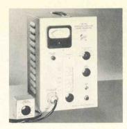
Type 190 Constant-Amplitude Signal Generator is ideal for checking amplifier high-frequency response. It generates sine waves over the range of 350 kc to 50 mc, continuously variable. Output amplitude at the cable termination varies less than 2% from 350 kc to 30 mc; less than 4% to 50 mc. Amplitude is continuously variable from 4 mv
