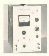
Type 105 Square-Wave Generator is continuously variable over the frequency range of 25 cycles to 1 mc. Risetime is 0.02 µsec when the output is terminated in a resistive load of less than 100 ohms. Direct-reading frequency meter is accurate within 3% of full scale. Output amplitude—0 to 100 v maximum, 0 to 15 v across 93 ohms. Sync amplitude control per-
