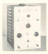
**Type 104A Square-Wave Generator** is a low-cost source of square waves for testing wide-band amplifiers, filter networks, and attenuator circuits in the laboratory or on the production line. The Type 104A generates four fixed frequencies: 50 cycles, 1 kc, 100 kc, and 1 mc. Risetime of the two high frequencies is 0.02 μsec; the two low frequencies, 3μsec. Amplitude of
