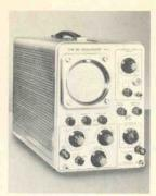
Type 310 Oscilloscope is a dc to 4 mc portable precision instrument, designed for both field and laboratory applications. With its small size...10"h by 634" w by 17"d... and its light weight, only 23½ lbs... the Type 310 handles easily and fits into tight spots, yet it is fully capable of performing much of your laboratory work.
