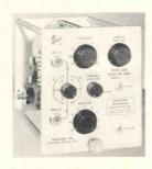
Type 53G Differential Wide-Band DC Unit—DC to 10 mc, 0.035-µsec risetime with Types 531 and 535 . . . dc to 5 mc, 0.07-µsec risetime with Type 532. Sensitivity 0.05 v/cm to 20 v/cm in 9 calibrated steps, 0.05 v/cm to 50 v/cm continuously variable. Separate step attenuators for both inputs. Rejection is better than 100 to 1 at full gain for the entire passband, 300 to 1 at 60 cycles. Weight 4½ lbs. Price \$175.
