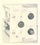
**Type 53A Wide-Band DC-Coupled Unit**—dc to 10 mc, 0.035-μsec risetime with Types 531 and 535...dc to 5 mc, 0.07-μsec risetime with Type 532. Sensitivity 0.05 to 50 v/cm, ac or dc, continuously variable, with 9 calibrated steps from 0.05 to 20 v/cm. 80 db isolation between two input connectors. Weight 3½ lbs. Price \$85.
