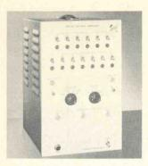
Type 180 Time-Mark Generator is a source of time markers, sine waves, and trigger impulses. Time markers of 1, 5, 10, 50, 100, 500 microseconds—1, 5, 10, 50, 100, 500 milliseconds—1 second, are available separately and simultaneously through pin jacks at 20 to 50 v, or mixed in any combination through uhf connector at 1 to 3 v. Sine waves of 5 mc, 10 mc, 50 mc
