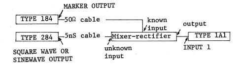
Set the TYPE 184 MARKER SELECTOR to  $10\mu s$ . Set the TYPE 284 SQUARE WAVE AMPLITUDE to 100 mV, the PERIOD to  $10\mu s$  and the MODE to SQUARE WAVE OR SINE WAVE OUTPUT.
