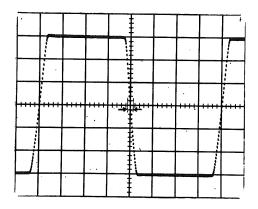
It may be necessary to adjust R31 so that the duty factor of the  $10\mu s$  period is not exactly 50% in order to bring the duty factor of all three periods within limits.
