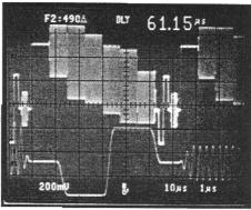
The 2467BHD automatically triggers on trilevel sync pulses used in high-definition video signals. Note: Line Count Readout Displays Field 2 – Line #490.
