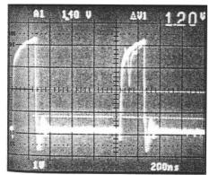
Metastability in this flip-flop occurs only once in a million normal cycles, yet it is clearly visible due to the 2467B's high visible writing speed.
