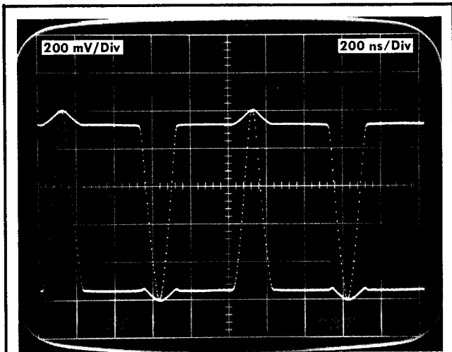
(A) Double-triggered, < unity loop gain
