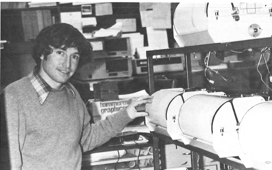
Figure 7. Drums at the Geophysics lab record analog signals picked up and communicated from 11 stations around the State of Kansas. Shlomo Shmuelov checks for traces that would indicate an earthquake.
