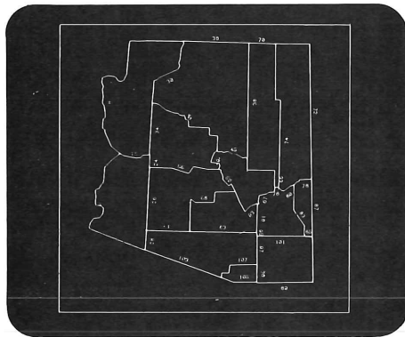
Figure 1. A map of the counties of Arizona encoded as polylines. The numbers appearing adjacent to the lines are the object ID numbers assigned by the system.
