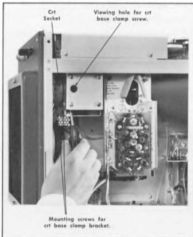
Fig. 4-3. Loosening the crt base clamp.
