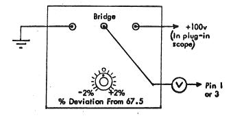
Set the dial on the 67.5 volt bridge to 67.5V and the multimeter to the most sensitive DC volts scale.
