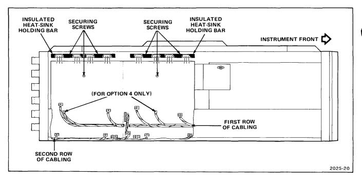
Fig. 7-6. A1-Deflection Amplifier board removal and replacement.
