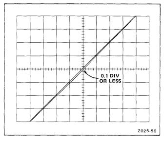
Fig. 4-5. Typical horizontal and vertical phase difference display.
