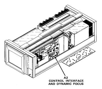
Fig. 10-5(A). Location of A2 Control Interface and Dynamic Focus board.
