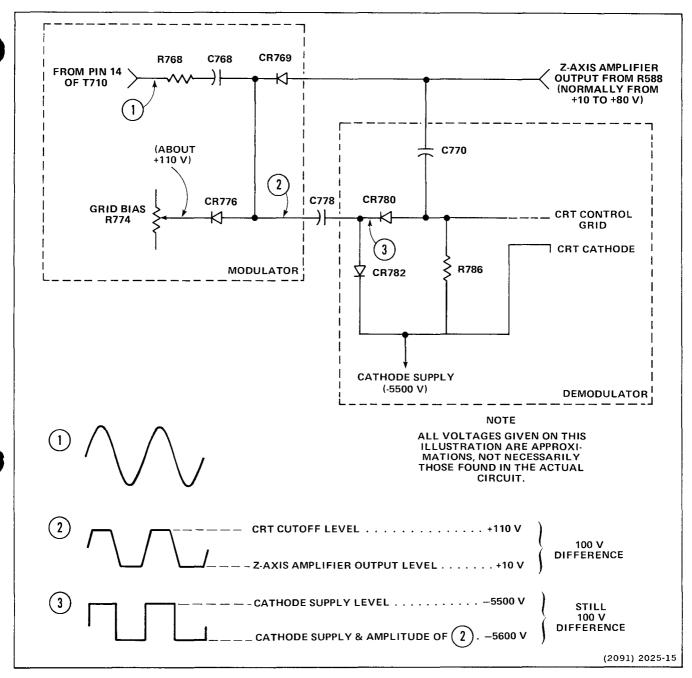
Fig. 6-5. Simplified diagram of the Control-Grid Dc Restorer.
