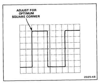
Fig. 4-3. Typical crt display for adjustment of vertical (Y) compensation and output gain.
