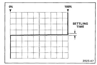
j. ADJUST—C330 (-X Atten Comp) for an optimum square corner on the 606A display.
