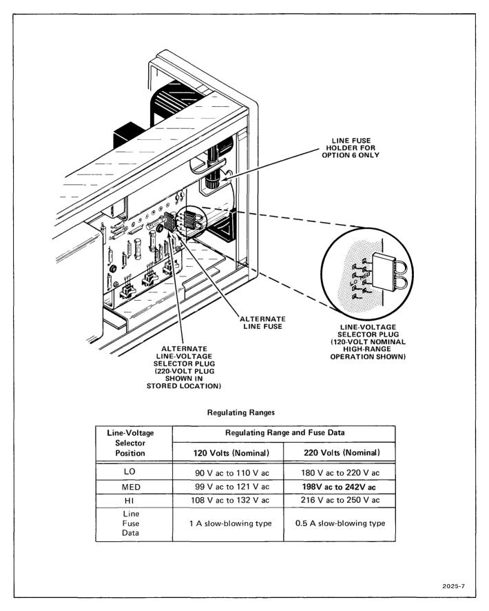
Fig. 5-1. Location of line-voltage selector plugs, regulating-range pins, and line fuses.
