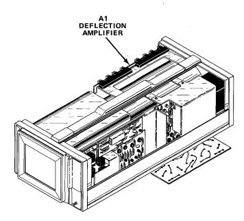
Fig. 10-2. A1-Vertical (Y) Amplifier component and waveform test point locations.
