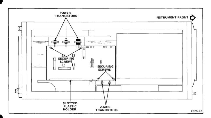
Fig. 7-7. A4—Low-Voltage Power Supply and Z-Axis board removal and replacement.
