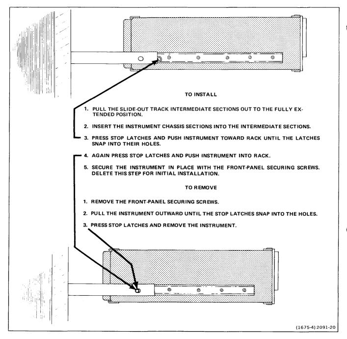
Fig. 5-3. Installing and removing a rackmounted instrument.
