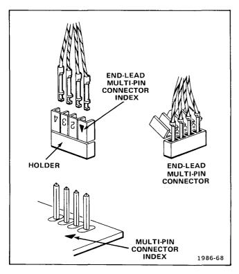
Fig. 7-3. Orientation of multi-connector holders.
