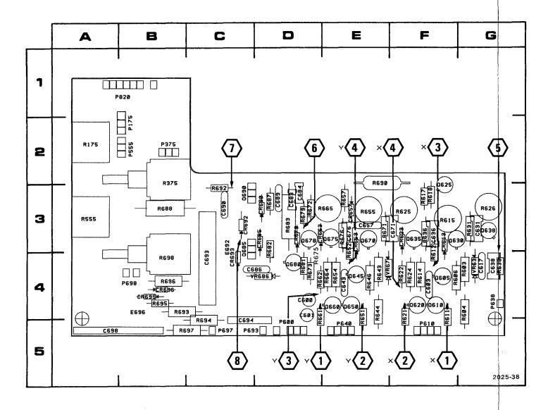
Fig. 10-5. A2-Dynamic Focus component and waveform test point locations.
