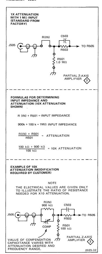
Fig. 5-2. Typical method for modifying Z-Axis input impedance and attenuation.
