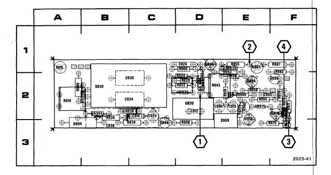
Fig. 10-8. A5-Sweep (Option 4) component and waveform test point locations.
