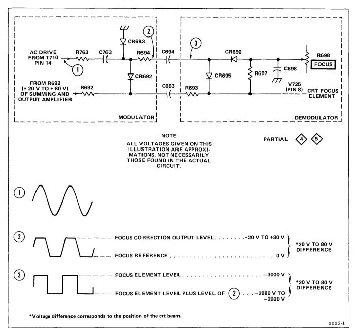
Fig. 6-4. Simplified diagram of Focus-Element Dc Restorer.
