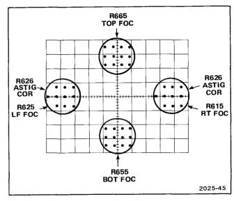
Fig. 4-6. Focus and astigmatism correction adjustments corresponding to the appropriate area of the dot display.
