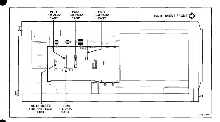
Fig. 7-4. Location and rating of power-supply fuses.
