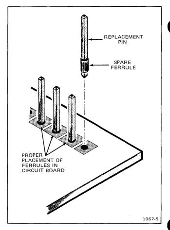
Fig. 7-8. Exploded view of circuit-board pin and ferrule.
