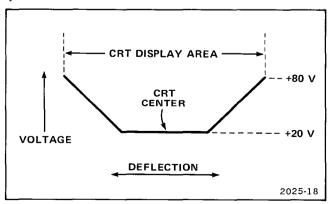
Fig. 6-3. Typical correction-voltage curve applied to the crt focus element (correction voltage applied for both vertical and horizontal deflection).
