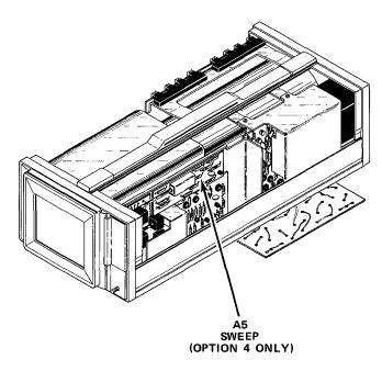
Fig. 10-8(A). Location of A5 Sweep board.
