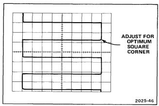
Fig. 4-1. Typical crt display for adjustment of horizontal (X) compensation and gain.
