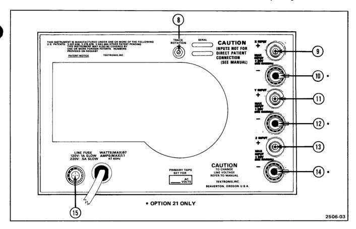
Fig. 2-2. Rear-panel controls and connectors (includes Option 21).
