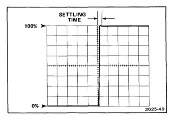
Fig. 4-4. Typical crt display for vertical settling time measurement (settling time includes corner distortion).
