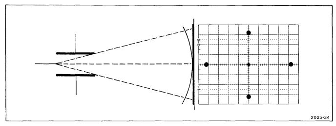
Fig. 6-2. Simplified illustration of geometric defocusing.
