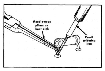
Fig. 7-5. Use of a heat sink to protect components during soldering.
