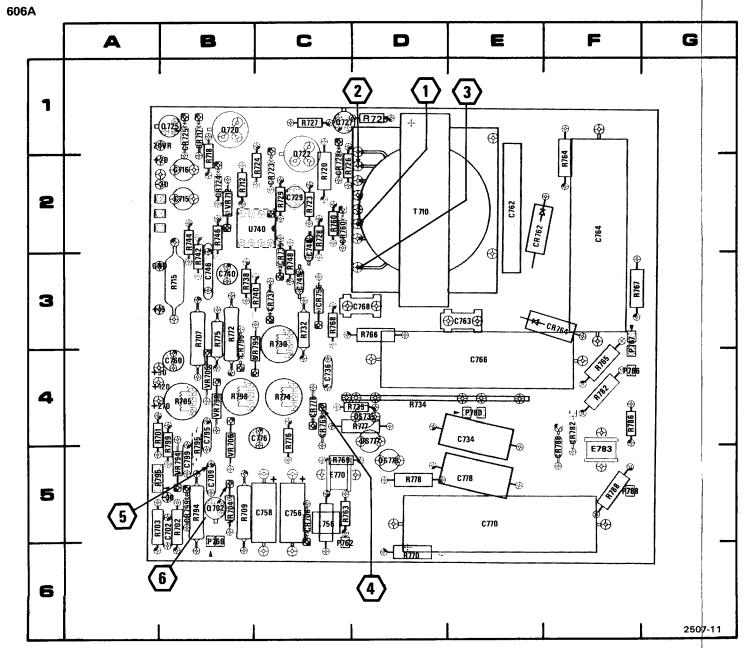
Fig. 10-6. A3-High-Voltage Power Supply component location and waveform test point locations.
