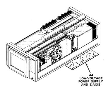
Fig. 10-7. Low-Voltage Power Supply component locations.
