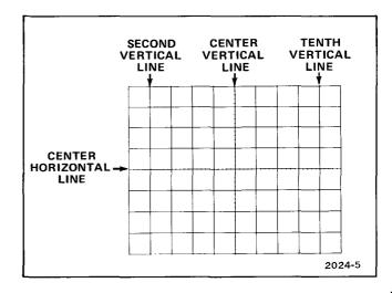
Fig. 2-3. Measurement lines on the 606A graticule.
