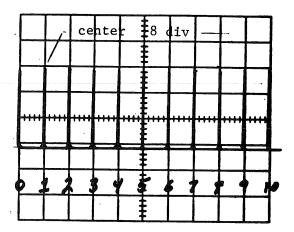
Sweep accuracy is checked over the center 8 div. Tolerances are distance between 9th time mark and number 9 graticule line. When the 1st time mark is aligned with the number 1 graticule line.
