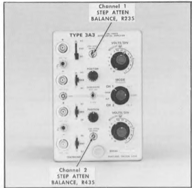
Fig. 6-3. Location of channel 1 STEP ATTEN BALANCE control, R235 and channel 2 STEP ATTEN BALANCE control, R435.
