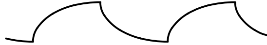
(b) Low-Frequency Information from Hall Device, Amplified and Applied to Input of Attenuator
