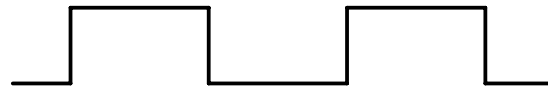
(d) Resultant Waveform Seen at the Output of the AM 503A—a Combination of (b) and (c)
