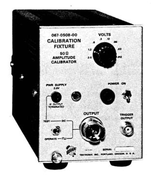
This calibrator provides a source of voltage, the overall accuracy of which is  $\pm 0.25\%$ , from an accurate 50 ohm source resistance to calibrate equipment having a characteristic 50 ohm impedance. It may also calibrate a high impedance input provideed the unit is accurately terminateed in total load of 50 ohms.
