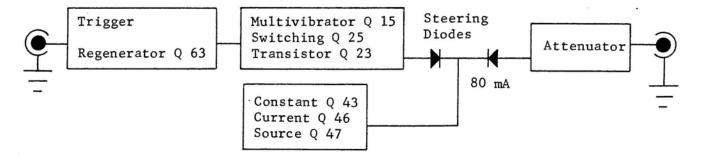
The 50  $\Omega$  Amplitude Calibrator consists of a precision constant current source, precision 50  $\Omega$  termination, an attenuator, and a switch.
