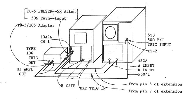
Adjust the bias on the TYPE TU-5 pulse to the firing level. Change the TYPE 5T3 TRIG SOURCE to EXT and adjust the TRIG LEVEL for a triggered display. Use the TYPE 10A2A POSITION control to center the display on the graticule area. Adjust equally between the TYPE 4S2A CH A and CH B MILLIVOLTS/CM VARIABLE controls for a 5cm display. Adjust the TYPE 11B2 DTM and TYPE 5T3 TIME POSITION to display the leading edge of the waveform.
