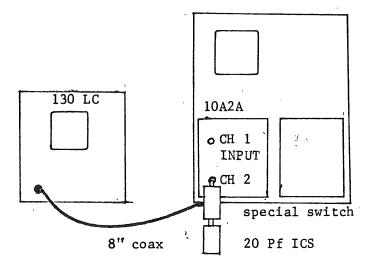
Set the switch to STD and the TYPE 130 RANGE SELECTOR to  $3\mu\mu F$ . Adjust the TYPE 130 COARSE and FINE ZERO for a mid scale meter reading. Change the switch to UNK. The TYPE 130 meter reading must stay within 6 minor div of mid scale at each position of the TYPE 10A2A VOLTS/CM switch and with the input selector in DC and AC. Repeat the check for the other channel.
