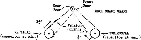
The full left (ccw) stop on the knob shaft is then set so the full left (ccw) rotation of the AMPLIFIER PHASING knob will be checked with the linkage in the illustrated position. The AMPLIFIER PHASING knob corresponding to 0 divisions on the front panel scale as illustrated below (left). Rotate the knob to indicate 100 divisions and set the other stop to check full right (cw) rotation at this point as illustrated below (right).
