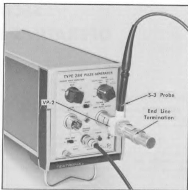
Fig. 2-2. S-3 probe - VP-2 connections.
