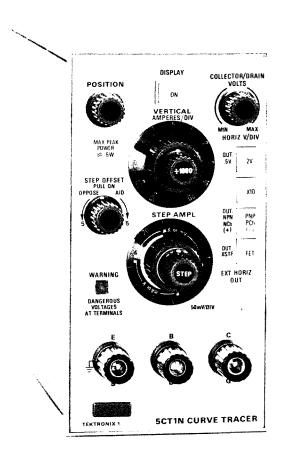
Fig. 1-1. 5CT1N Curve Tracer.
