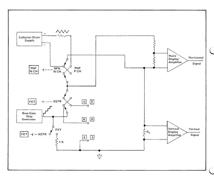
Fig. 2-1. Simplified block diagram of the 5CT1N.
