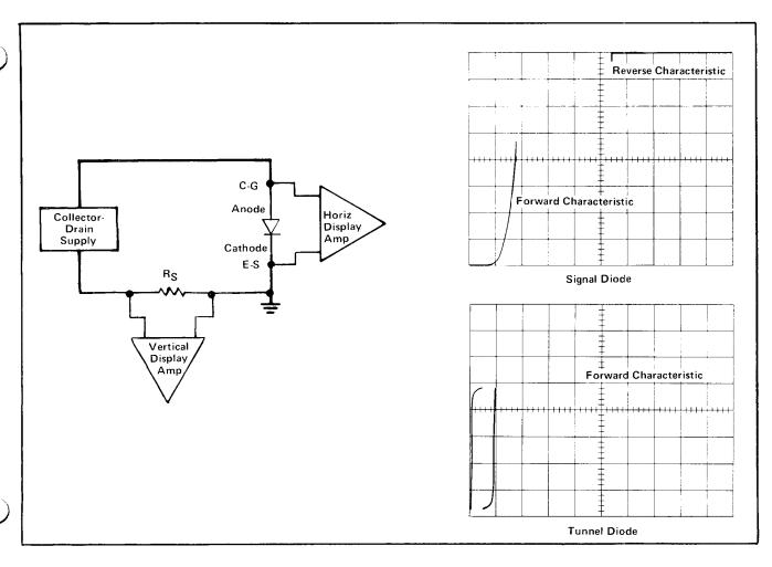
Fig. 1-4. Simplified diagram illustrating connection of diode to 5CT1N and typical displays.
