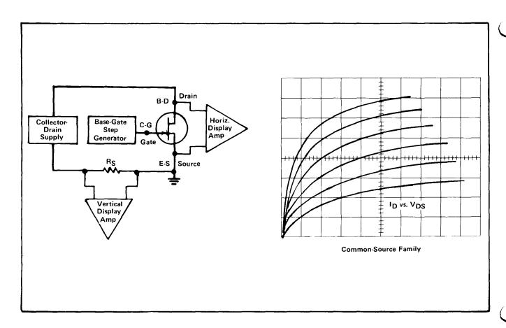
Fig. 1-6. Simplified diagram showing connection of FET to 5CT1N and typical display.
