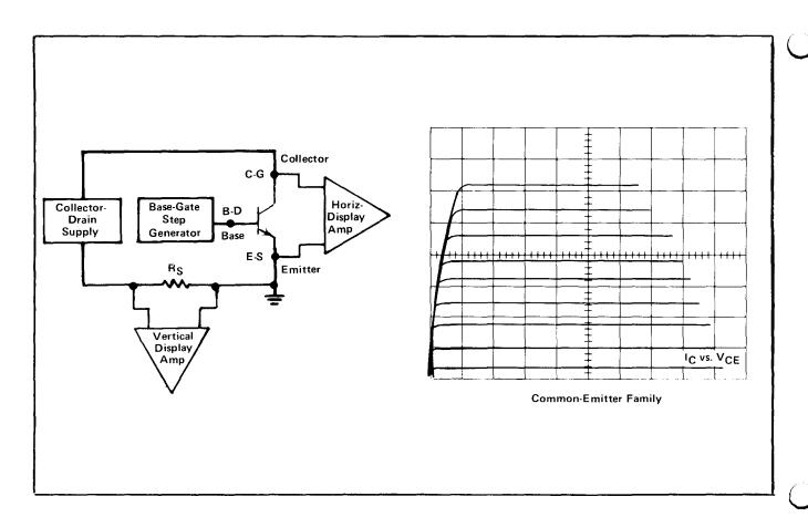
Fig. 1-5. Simplified diagram showing connection of Bipolar transistor to 5CT1N and a typical display.
