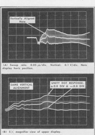
Fig. 6-9. 85 MHz test oscilloscope displays of Type S-2 double triggered output signal showing unity loop gain. TP121 or TP161, step 4.
