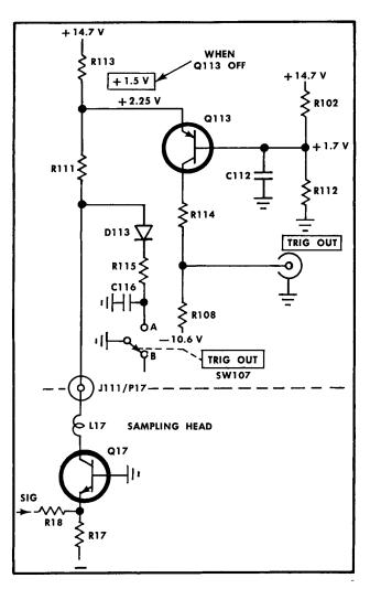
Fig. 4-2. Channnel B Trigger circuit connections.
