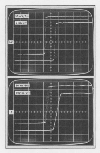
Fig. 2-8. Random sampling operation using TRIG OUT signal for Ext. triggering Type 3T2 (SN B010101-B040249).
