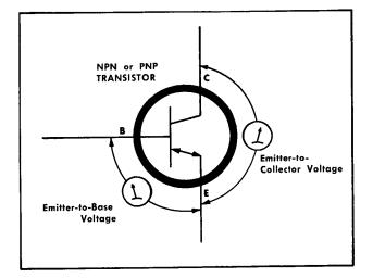
Fig. 5-5. In-circuit checks NPN or PNP transistors.
