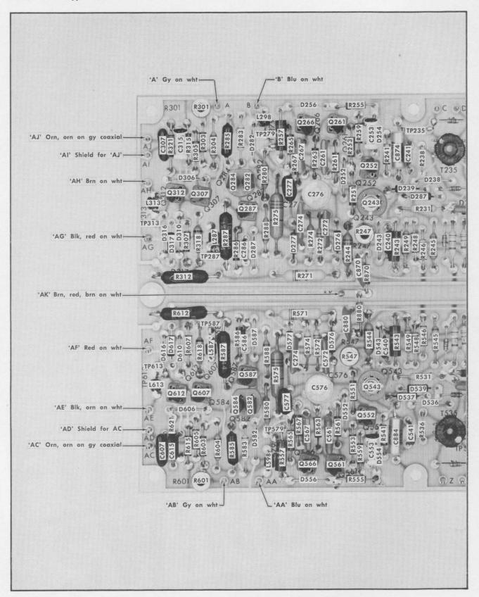
Fig. 5-8A. Vertical circuit board assembly, left.
