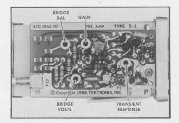
Fig. 6-10. Sampling Head adjustments, left side.
