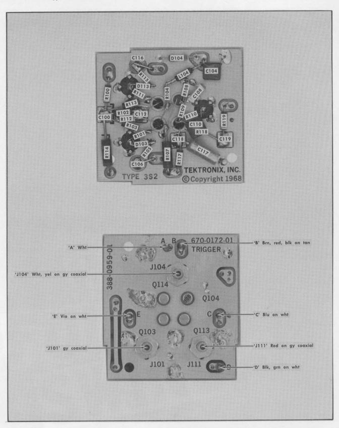
Fig. 5-10. Trigger circuit card assembly, SN B040250-up.
