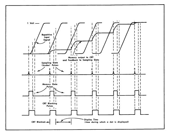
Fig. 3-3. Simplified representation of an error-sampled ratchet-memory waveform.
