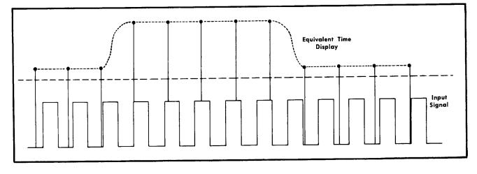
Fig. 3-1. Equivalent time display of repetitive real time signal by means of the sampling technique.
