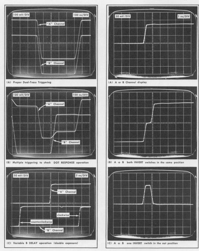
Fig. 2-4. Typical Displays to show dual trace operation.
