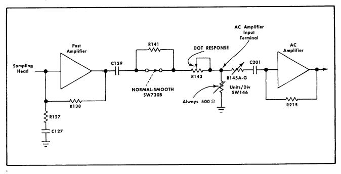
Fig. 4-3. Forward Attenuation network, showing that the output resistor of the Units/Div Forward Attenuator is actually the AC Amplifier input resistor.
