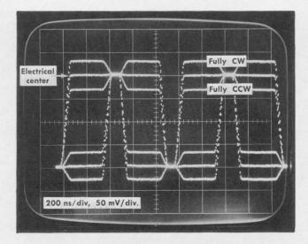
Fig. 6-12. Finding electrical center of Type 352 DOT RESPONSE control. Triple exposure; double triggered; 1 µs square wave.
