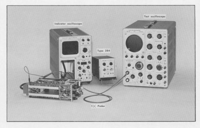
Fig. 6-3. Initial test equipment setup for steps 1 and 2.
