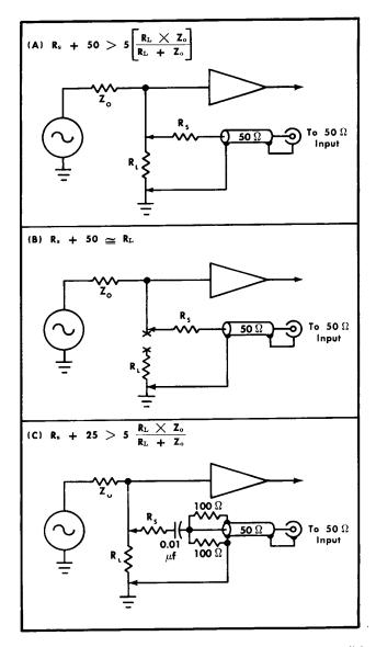
Fig. 2-14. Built-in probes for coupling to a test circuit. (A) Parallel method; (B) series method; (C) reverse-terminated parallel method.
