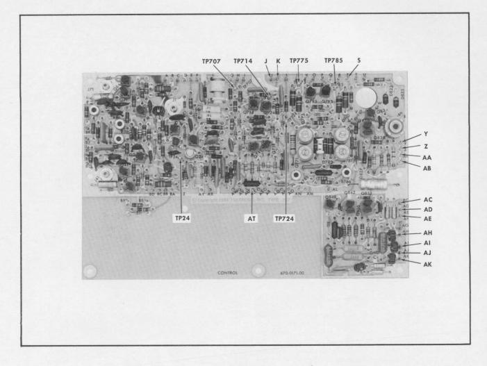
Fig. 5-4. Test point locations, Control circuit board.
