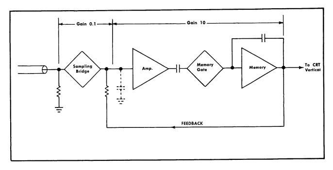
Fig. 3-2. Simplified block diagram of an error-sampled feedback system with a ratchet memory.
