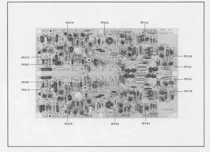
Fig. 5-3. Test point locations, Vertical circuit board.
