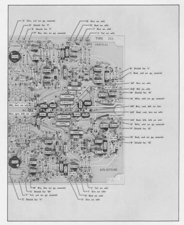
Fig. 5-8B. Vertical circuit board assembly, right.
