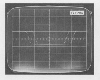
Fig. 2-12. Double triggered false display using a 100 ns period square wave.
