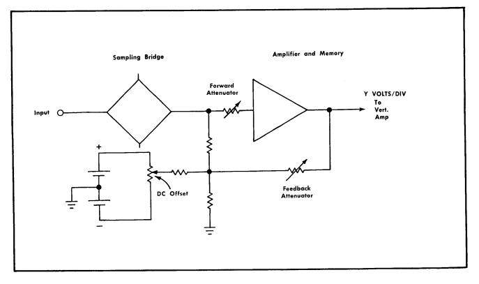
Fig. 3-7. Method of adding a DC Offset voltage to the memory feedback.
