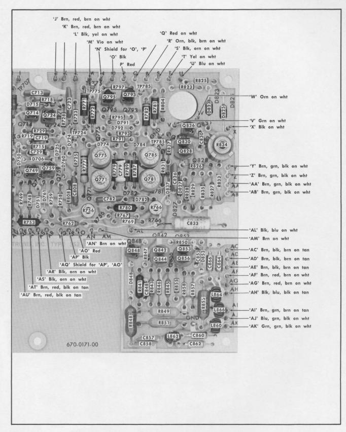
Fig. 5-9B. Control circuit board assembly, right.
