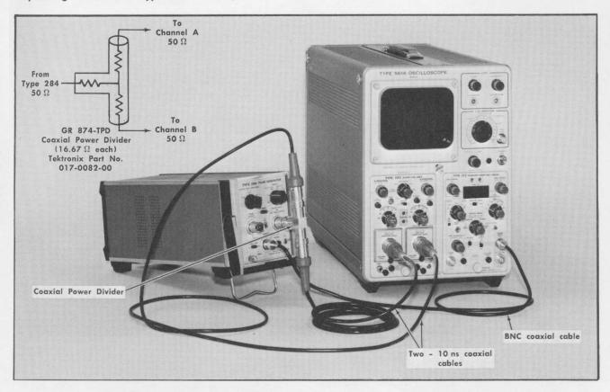
Fig. 2-3. Initial Power divider connections.
