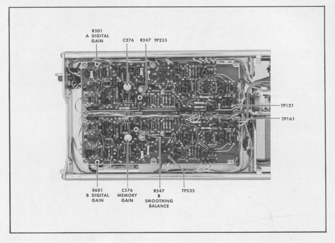
Fig. 6-6. Type 352 Left side test points and adjustments.
