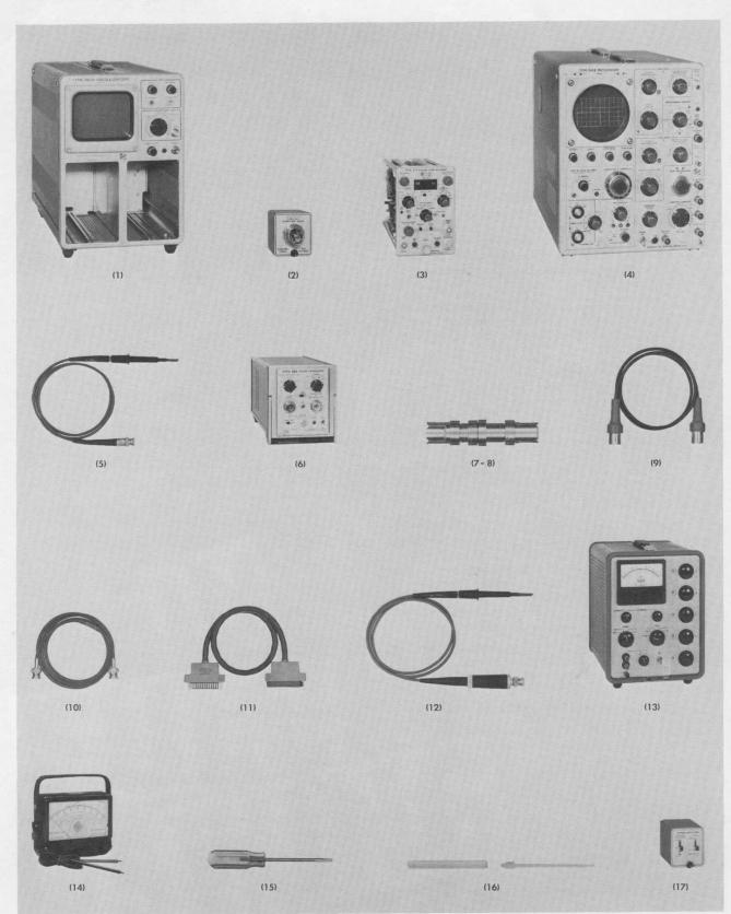
Fig. 6-1. Equipment required for Recalibration.
