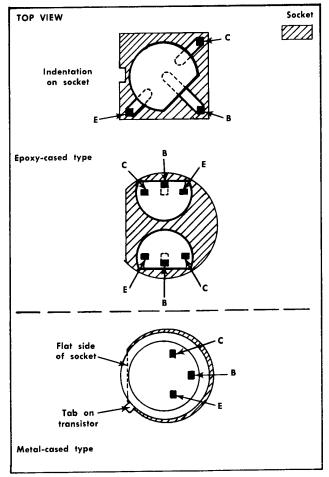
Fig. 5-6. Electrode configuration for socket-mounted transistors as viewed from the top of the transistor.
