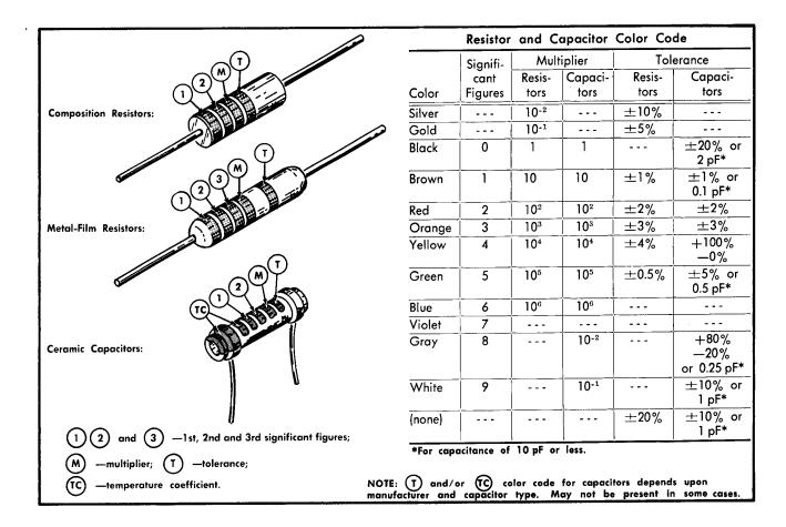
Fig. 5-1. Resistor and ceramic capacitor color-code.
