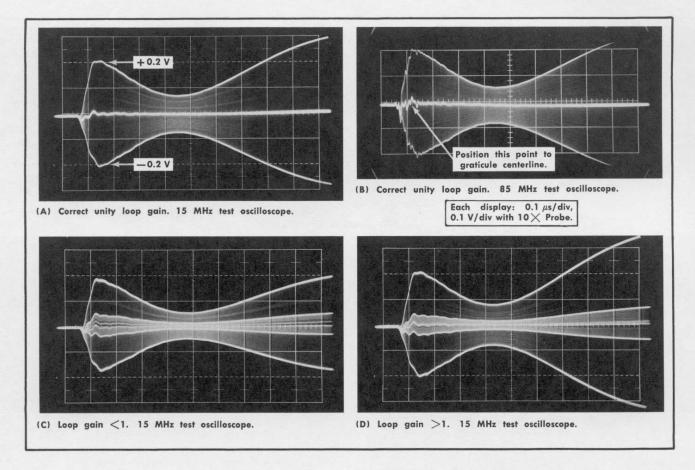
Fig. 6-8. Test oscilloscope displays of Type S-1 output signal (at TP121 or TP161) when externally triggered by Memory Gate signal. Timebase unit was double triggering on 1 μs period square wave.
