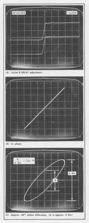
Fig. 2-6. A VERT B HORIZ operation including (A) initial setup (Dual Trace) (B & C), 500 MHz X-Y display.
