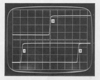
Fig. 6-13. Waveforms for step 17. Sweep rate: 2 ns/div, with Display mag switch at X1.
