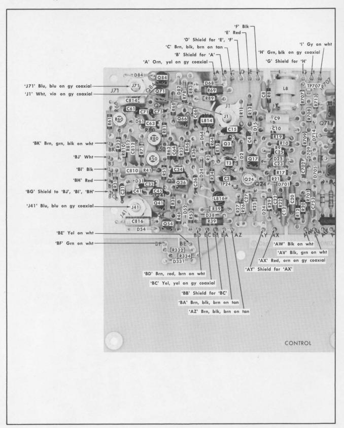
Fig. 5-9A. Control circuit board assembly, left.
