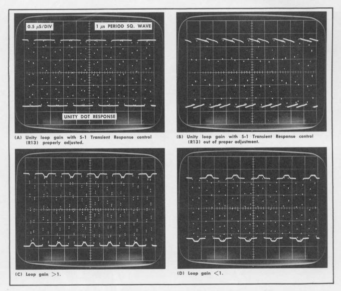
Fig. 6-7. Type 352/S-1 waveforms when signal is 1  $\mu s$  period square wave. Timebase was double triggered to show dot response.
